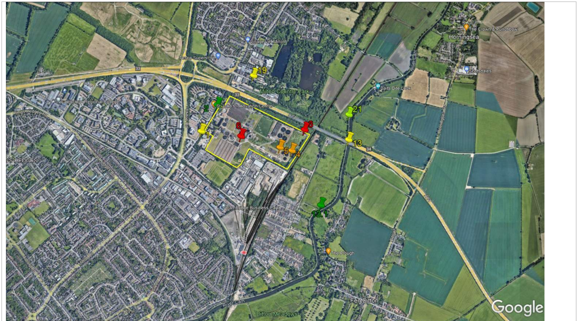
Figure 11: Sniff Survey 2 – Colour coded pins based on highest Odour Intensity Mean results for locations where ‘relevant’ odour(s) were detected
