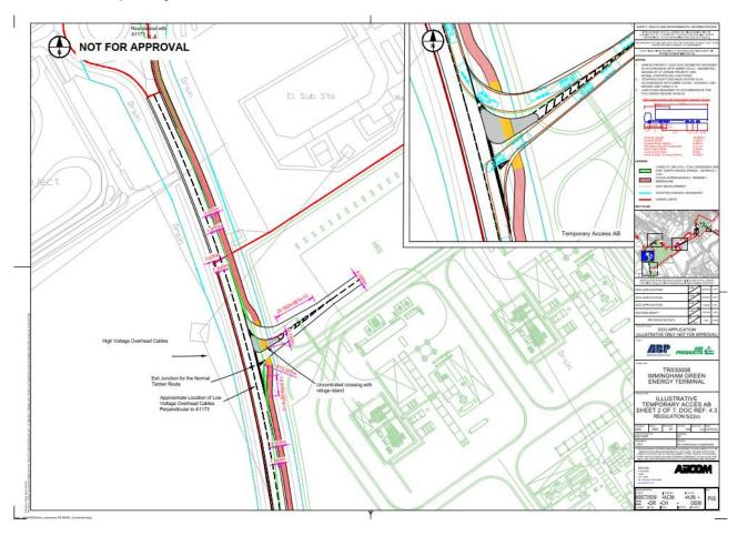
3.1.5 As can be seen in Plate 7, Temporary Access AB is a simple priority junction from the A1173 and has been designed to accommodate max legal HGV movements.
