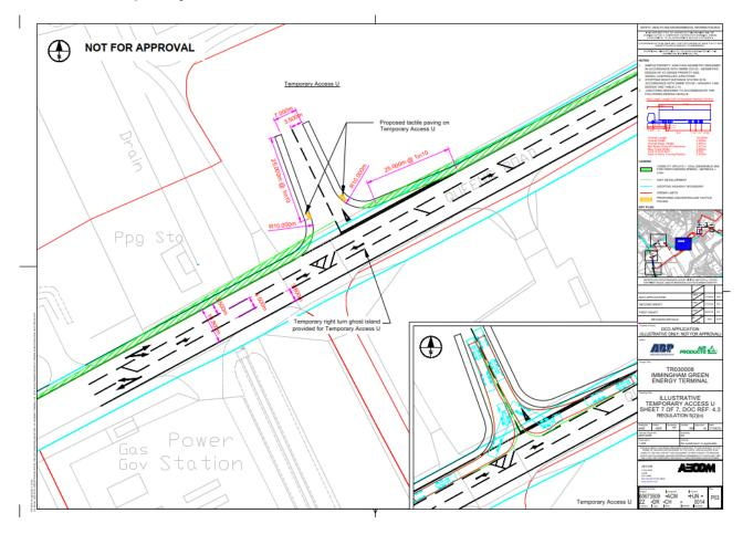
3.1.11 As can be seen in **Plate 12**, Temporary Access U is a right turn ghost island from Kings Road and has been designed to accommodate max legal HGV movements.
