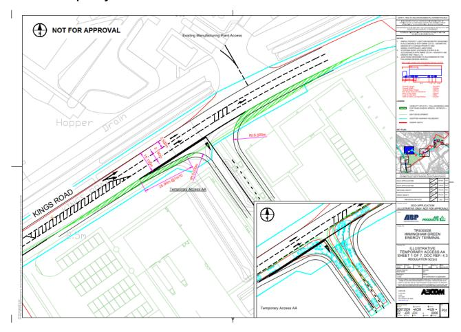
3.1.4 As can be seen in Plate 6, Temporary Access AA is a right turn ghost island from Kings Road and has been designed to accommodate max legal HGV movements.
