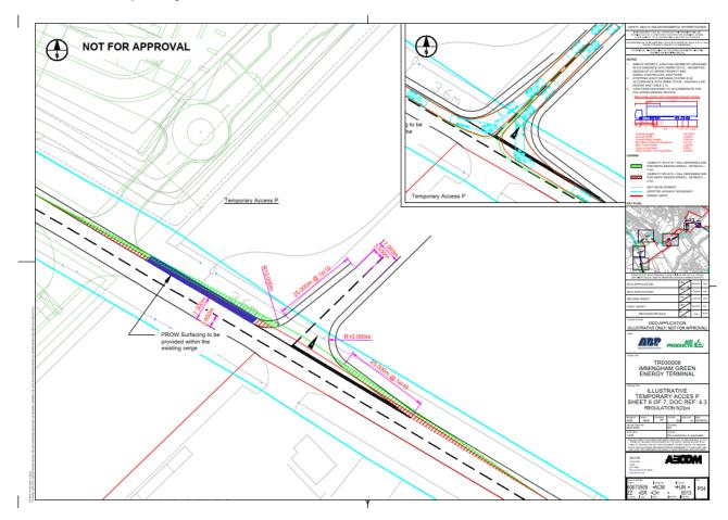
3.1.10 As can be seen in **Plate** 11, Temporary Access P is a simple priority junction from Laporte Road and has been designed to accommodate max legal HGV movements.
