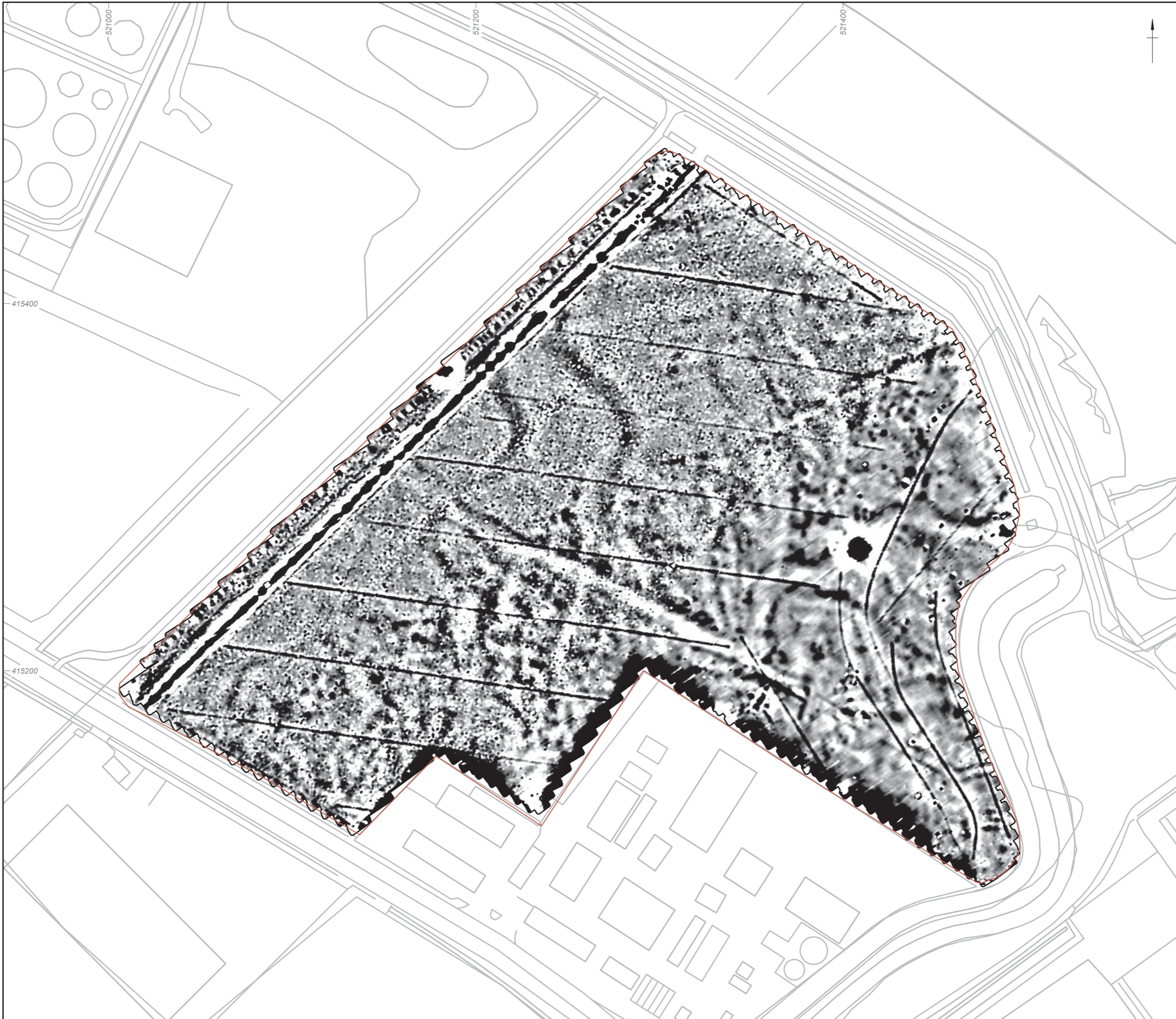
Figure 2: Detailed gradiometer survey greyscale plot
