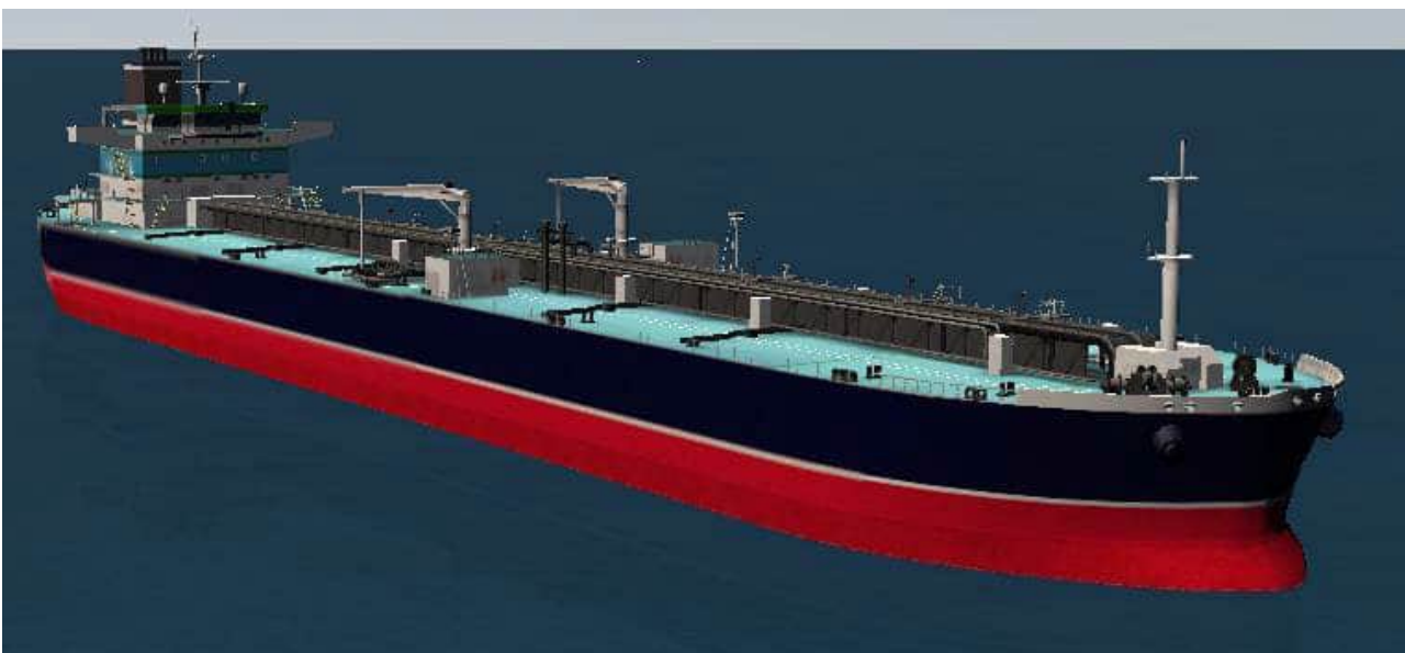
Figure 3.1: 243m x 42m products tanker ship manoeuvring model
