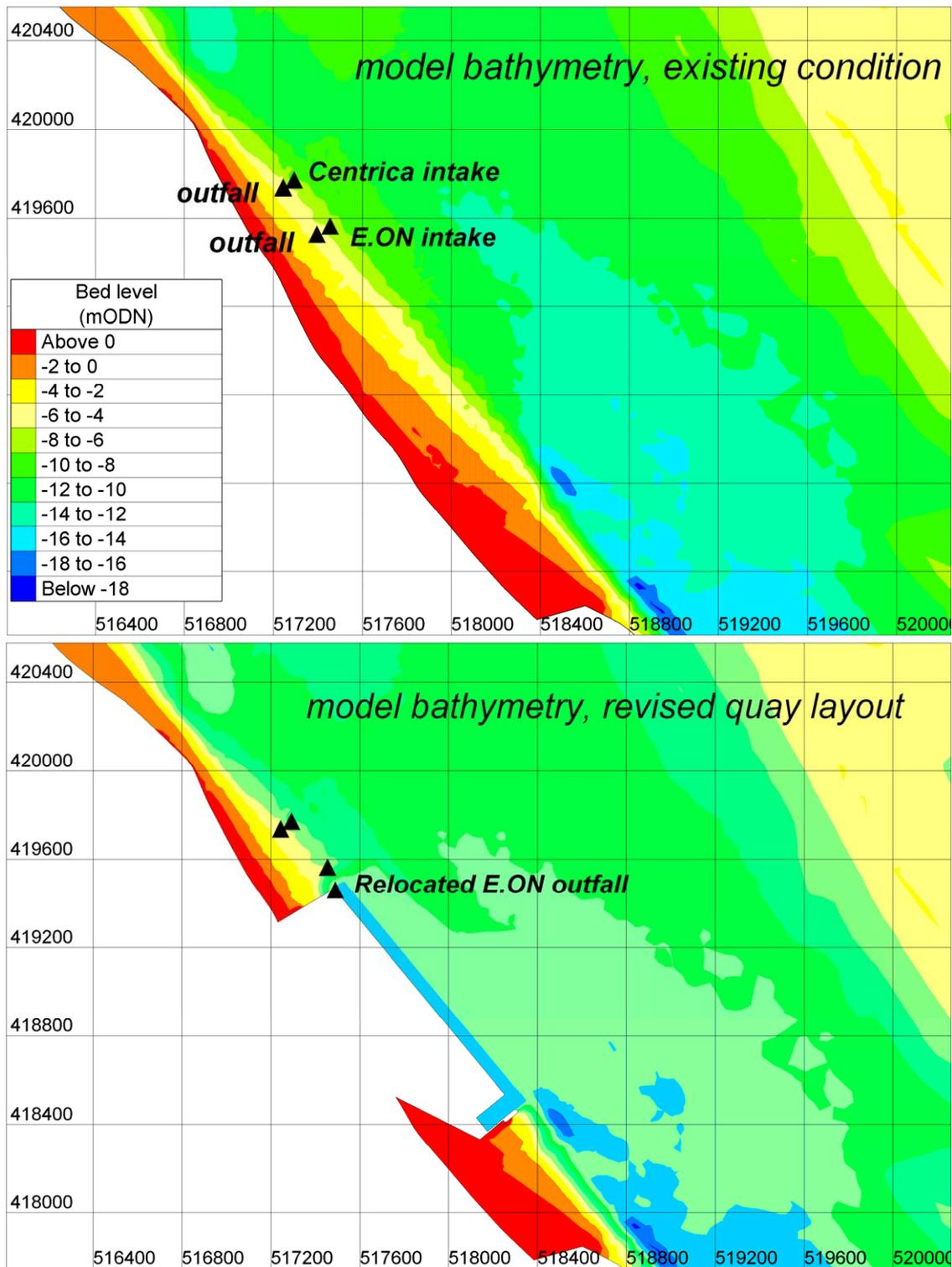
Figure 2.1 Site layouts; existing and revised developed case
