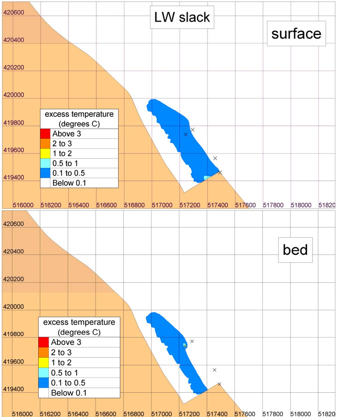
**Figure 2.3 Predicted thermal dispersion patterns at Low Water, final layout with E.ON outfall relocated, spring tide, calm conditions**
