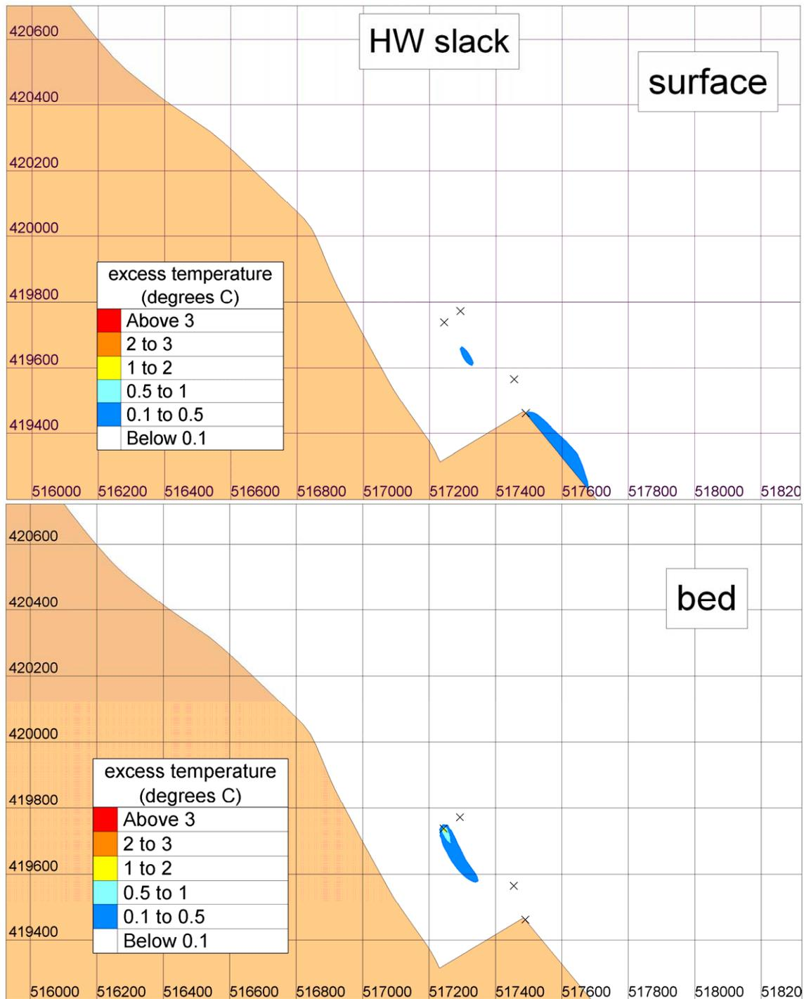
**Figure 2.2 Predicted thermal dispersion patterns at High Water, final layout with E.ON outfall relocated, spring tide, calm conditions**
