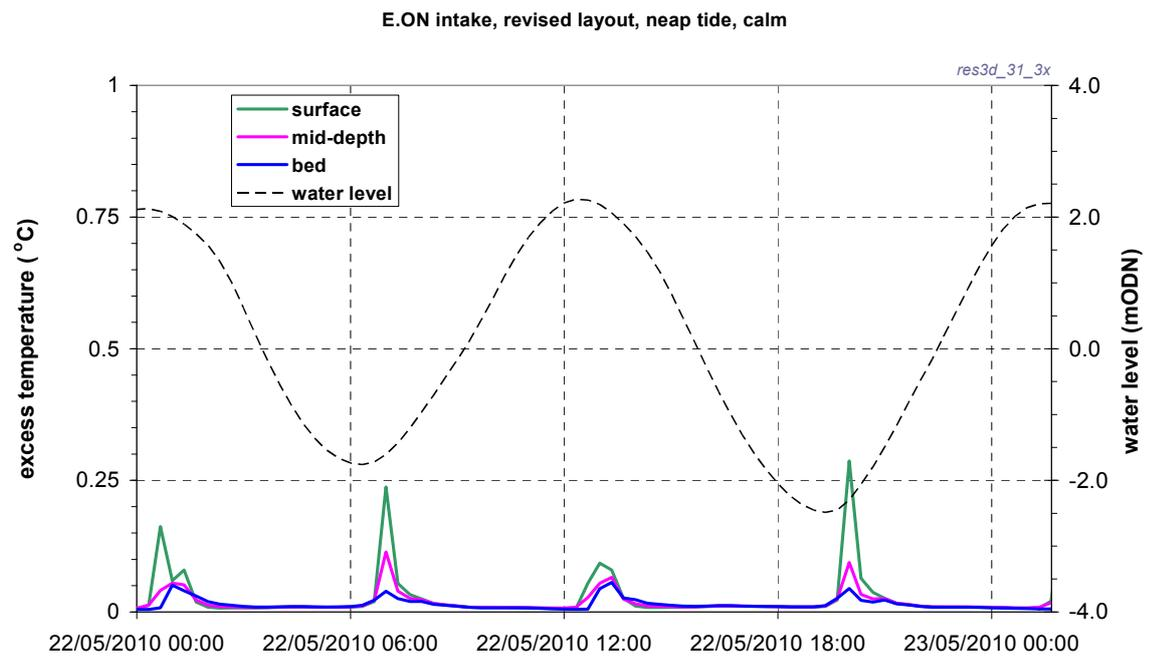
**Figure 2.5 Predicted excess temperature variation at the E.ON intake, final layout with E.ON outfall relocated, neap tide, calm conditions**
