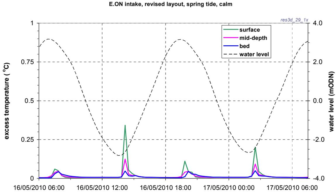
**Figure 2.4 Predicted excess temperature variation at the E.ON intake, final layout with E.ON outfall relocated, spring tide, calm conditions**
