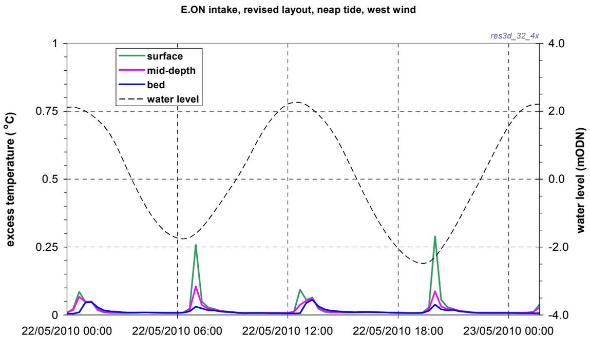
**Figure 2.7** Predicted excess temperature variation at the E.ON intake, final layout with E.ON outfall relocated, neap tide, constant wind
