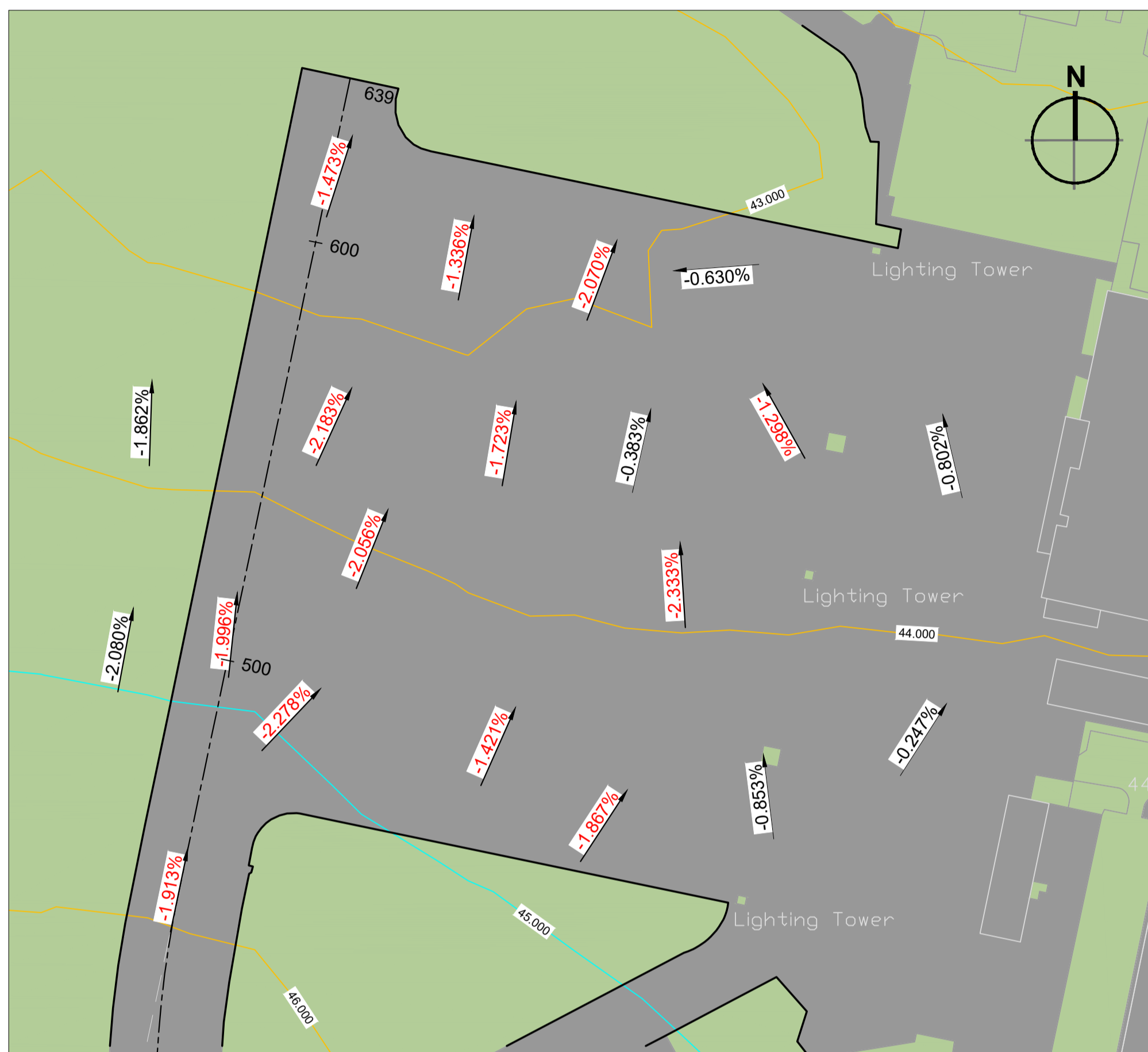
Passenger Terminal Apron - Non-compliance (clause E-360) On an aircraft stand, the maximum slope should not exceed 1% in any direction Scale 1:1000
