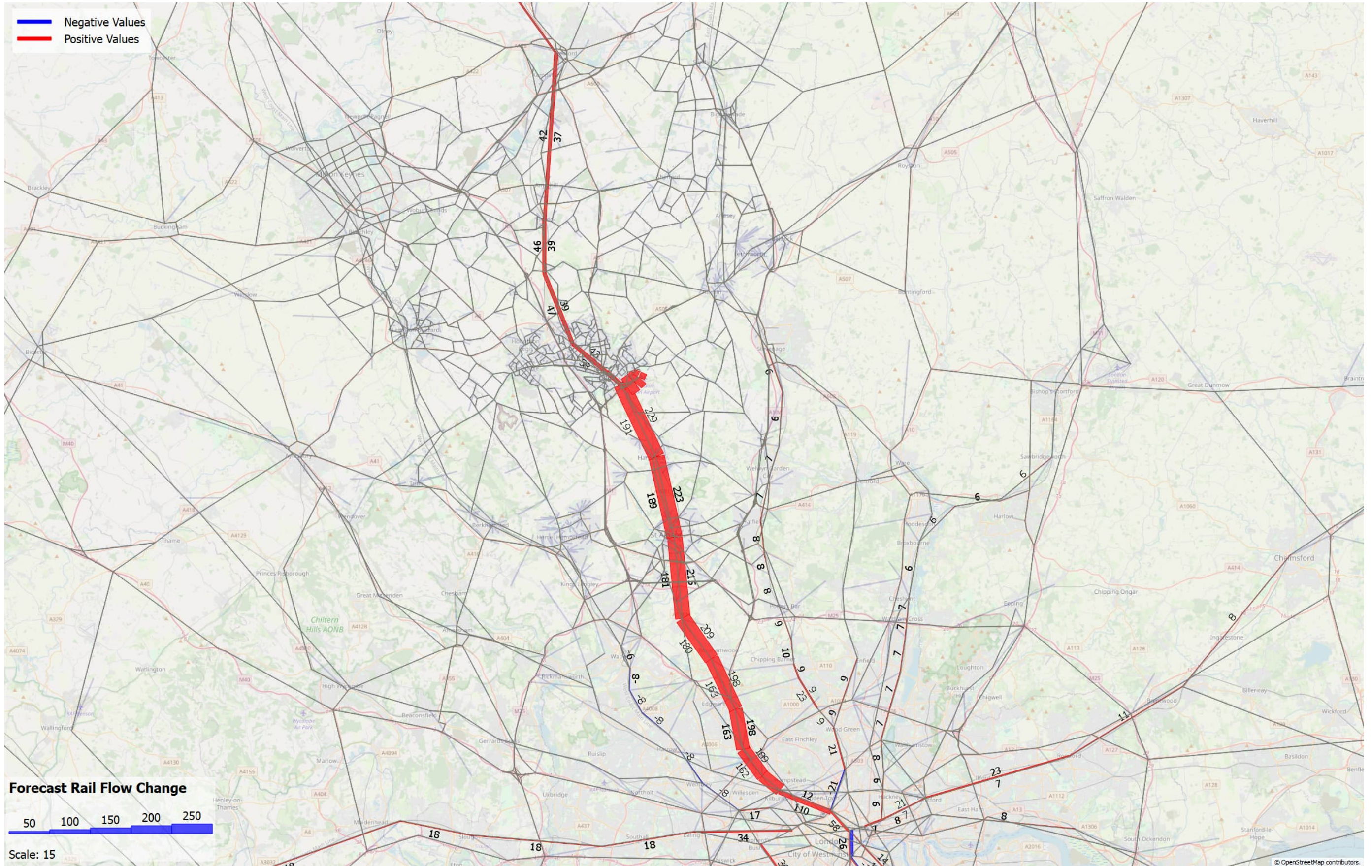
2039 PM Peak Updated Run "With" vs "Without" Expansion Rail forecast comparison (passenger per hour)
