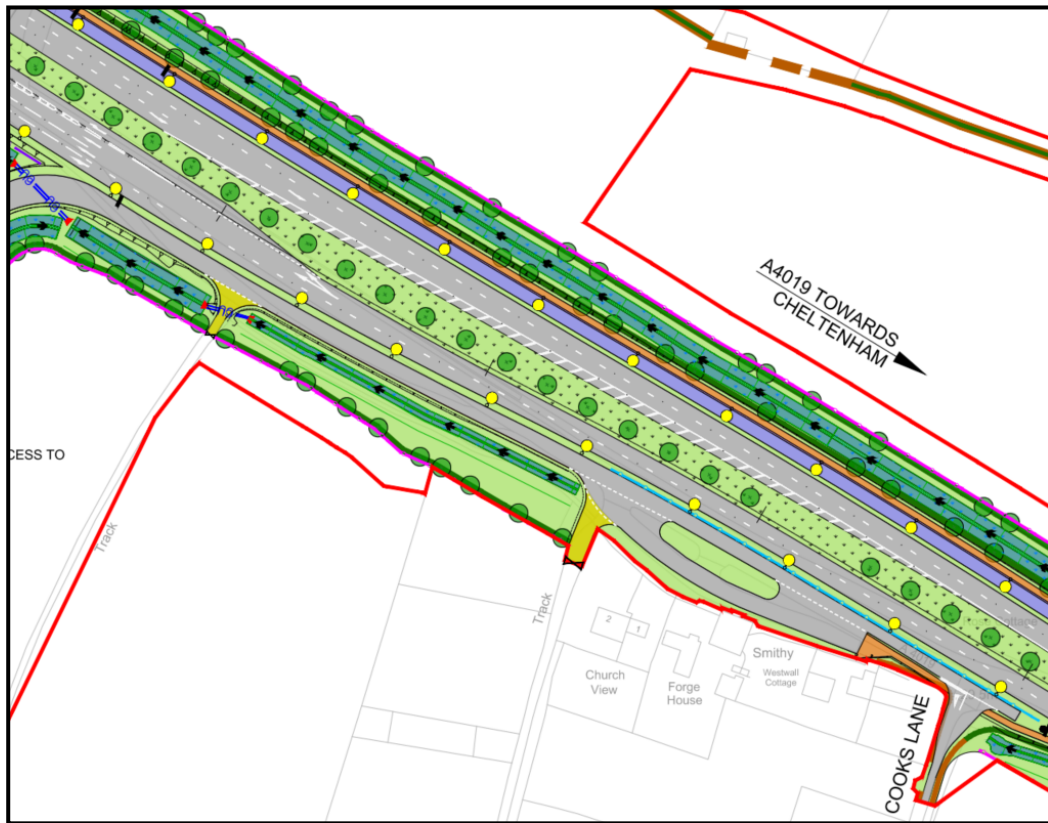
Figure 1-2 – Extract of General Arrangement Plan Showing Proposed Separation between Access Road and A4019
