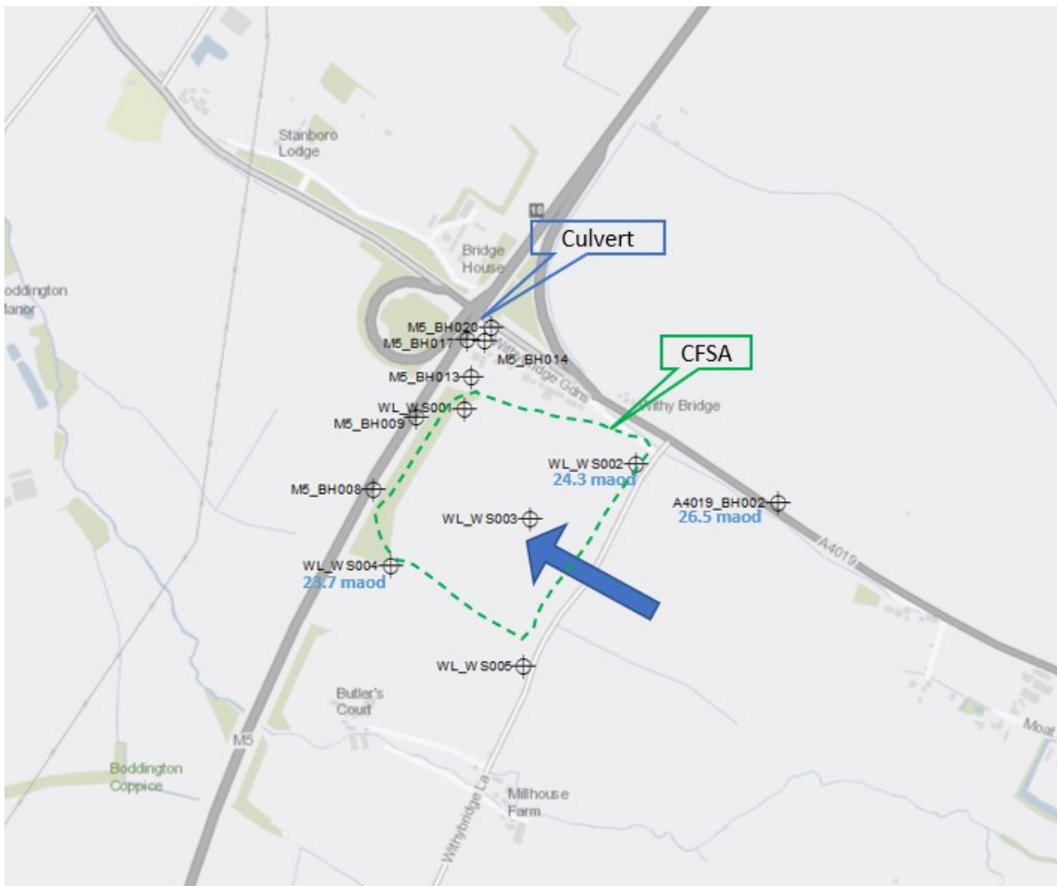
Figure 9 – Potential groundwater flow direction in the superficial deposits January 2022 (groundwater level shown in blue text)
