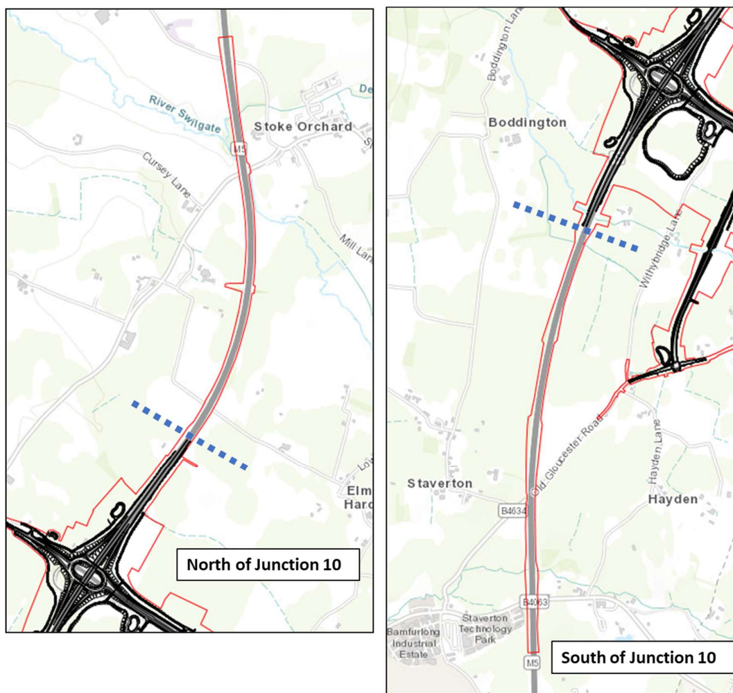
Figure 2-4 - Showing the sections of the M5 that are within the Order limits to the north and south of Junction 10, but do not include any highway alignment works. Scheme works within these areas are limited to the installation of new signage. The blue dashed lines denote the limits of the works on the slip roads, embankments and pavement.
