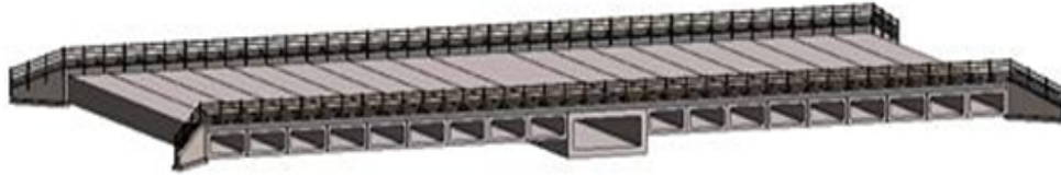
Figure 7-4 - Schematic of Proposed Northern Flood Culvert
