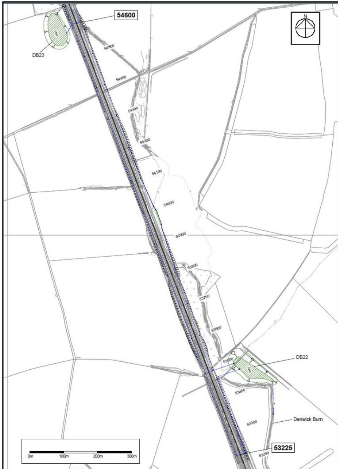
Figure 4-1 - Highway Drainage Layout and Detention Basin DB22
