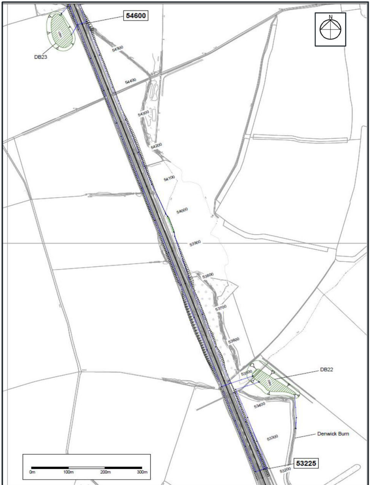
Figure 4-2 - Highway Drainage Layout and Detention Basin DB23
