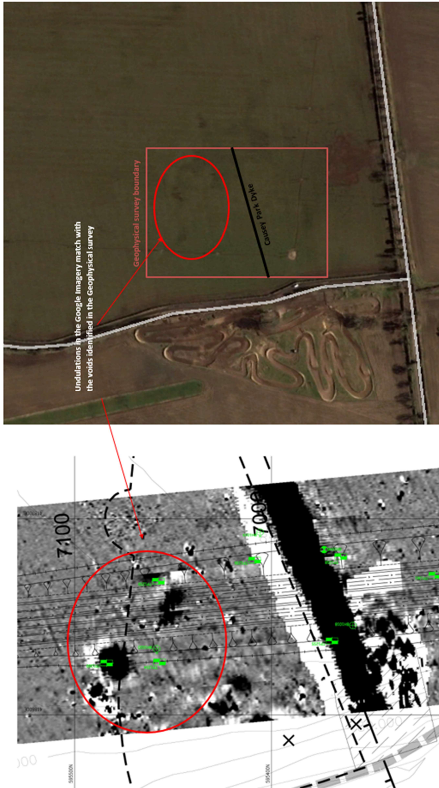
Figure 1-7 Geophysical Survey. Location of voids. Lang O'Rourke, Preliminary Geotechnical Report. 2006. Google Imagery 2018
