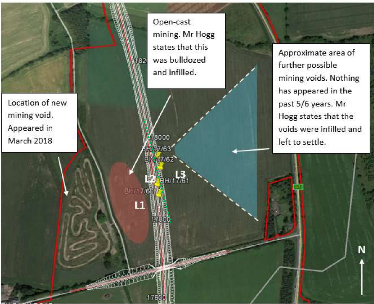
Figure 1-1 Location of historic mine features. Google Earth Imagery 2018
