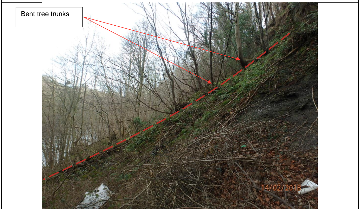
Photograph 2 – view east of the mid-slope, note the curved trunks of mature trees indicating the movement has been occurring for some time.
