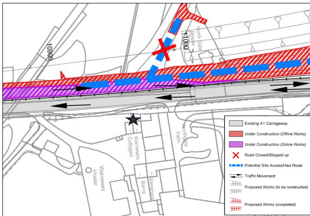
Figure A-1 - Phase 1 and 2 of Traffic Management Phasing Southern End (Warreners Cottages)
