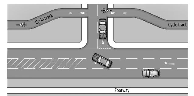
Figure E/4.9N Indicative layout of a bent-out crossing at a minor road
