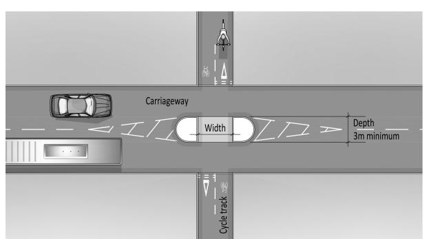
Figure E/4.6 Refuges at cycle traffic crossings
