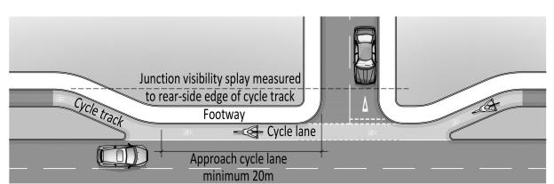
Figure E/4.16N2 Indicative layout of a bent-in crossing
