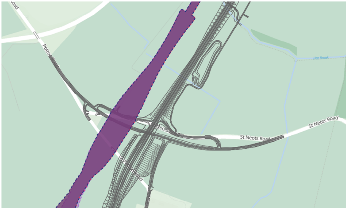
Figure 5 Potential engineering interaction between the Scheme and EWR Project Alignments 1,2 & 9 at B1046 / Potton Road
