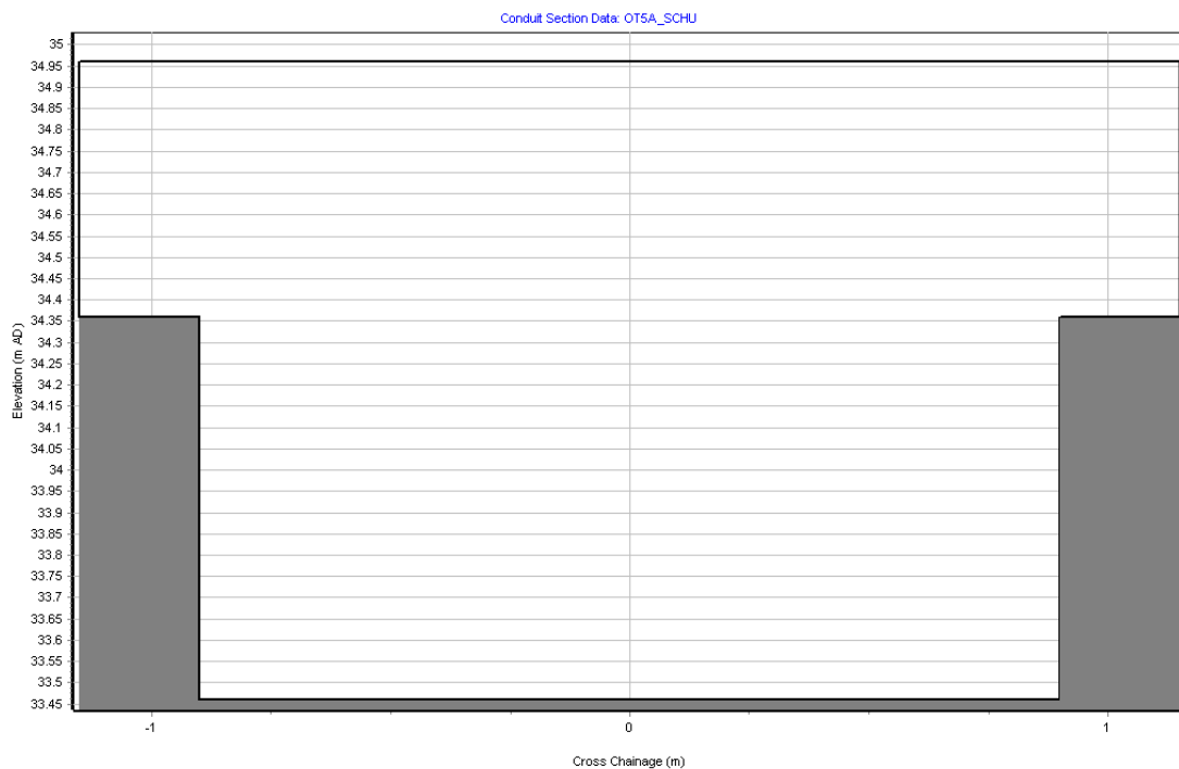
Figure 9-3: Top Farm Brook Proposed A428 Modelled Culvert
