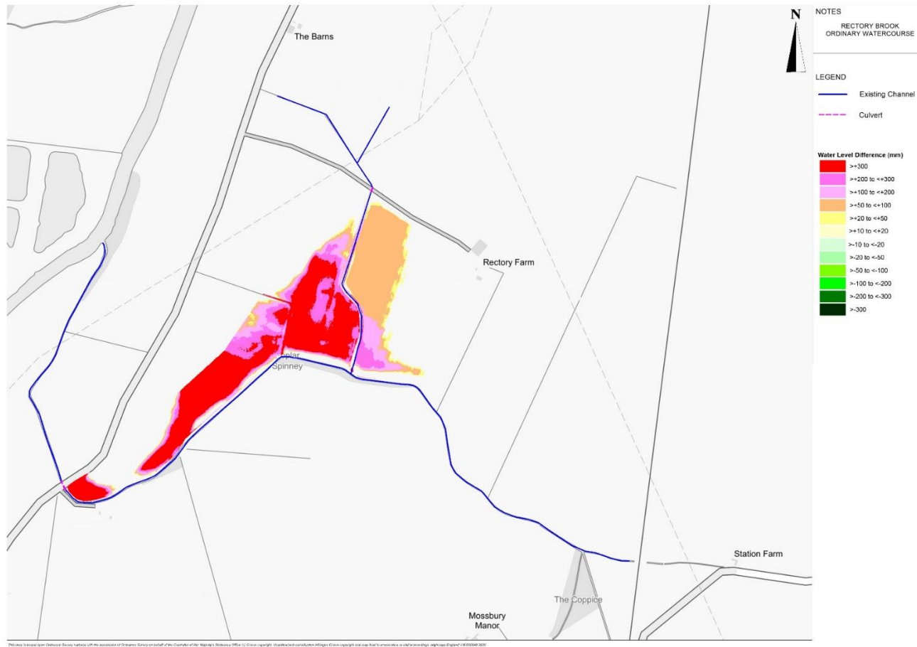
Figure 11-10: Depth Difference Map (Stone Brook 1% AEP & River Great Ouse 10% AEP Sensitivity) - 1% AEP + 65% Climate Change
