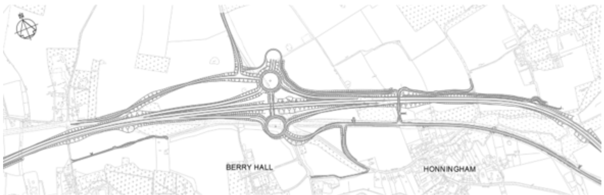
Figure 2-2: Scheme's Design of Wood Lane Junction
