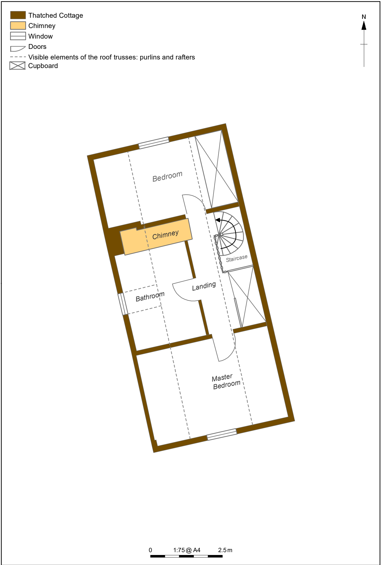
Figure 16: First floor plan, Thatched Cottage
