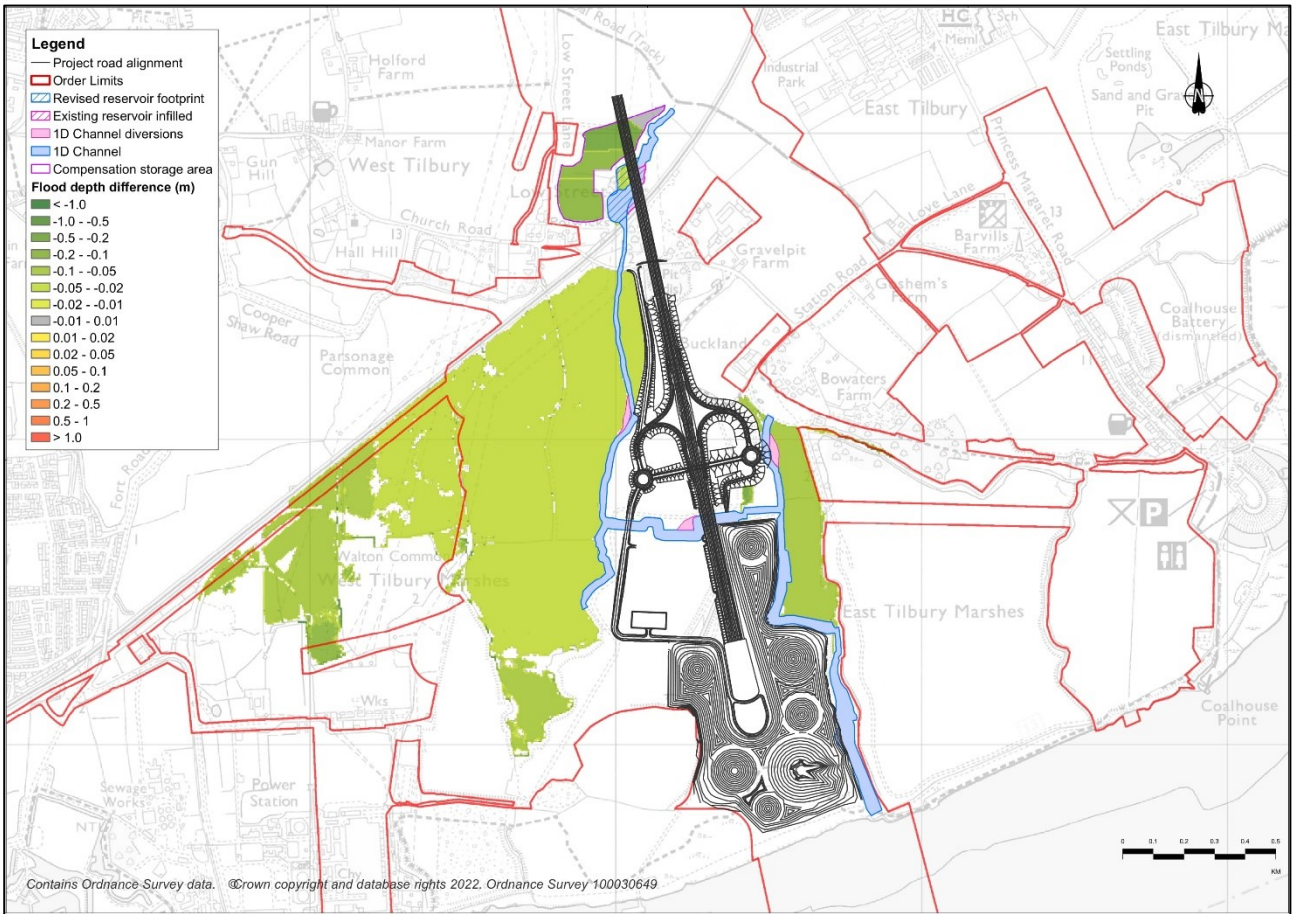
Plate 7.10 Maximum flood depth difference (-20% inflows minus post-development design simulation – 1 in 100 year fluvial event with 26% climate change allowance in 2130)
