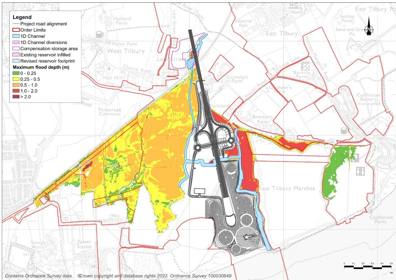
Plate 7.6 Maximum flood depth for post-development (without mitigation) design simulation – 1 in 1000 year fluvial event with 48% climate change allowance in 2130
