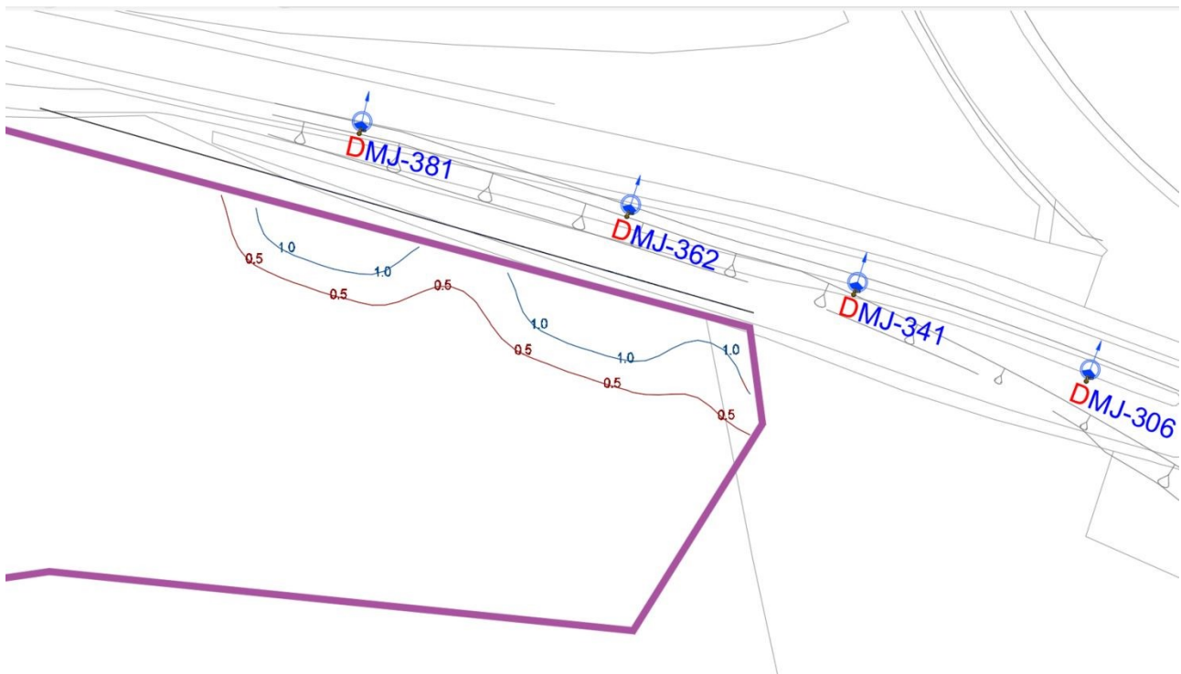
Plate 4.2: Close up view of light spill contours in key receptor area
