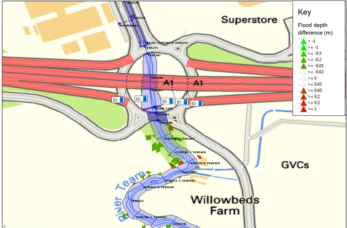
Figure 4-1 - Predicted flood difference between the existing and proposed scenarios for the 0.1% AEP event and the location of the proposed bridge pillars numbered 1 to 5 from east to west
