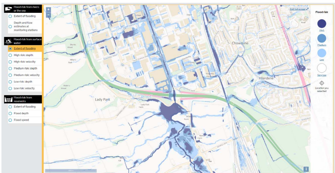
Figure 8 - Environment Agency's risk of flooding from surface water map centred on junction 67
