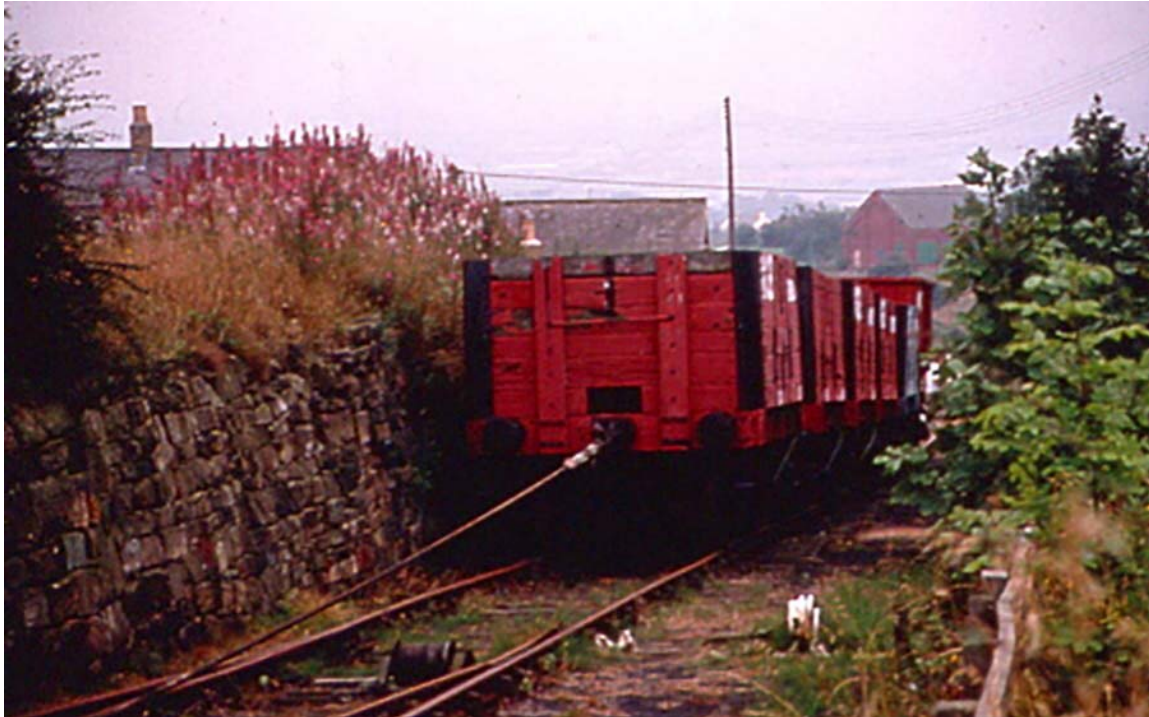
Image 1 – An example of one of the rope-hauled trucks on the Bowes Railway. The image also shows a masonry retaining wall flanking the track
