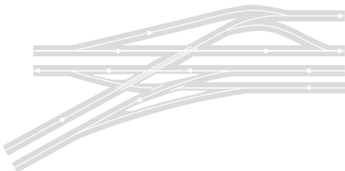
Figure A.14 3 leg 'Y' interchange of 2 motorways with mainline motorway and link roads
