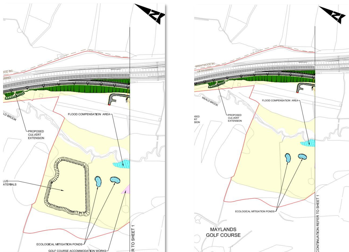
Figure 3.1 Scheme Layout Plans extracts from the Application (APP-010) (left hand side) and from proposed Change 1 (TR010029/EXAM/10.2) (right hand side)
