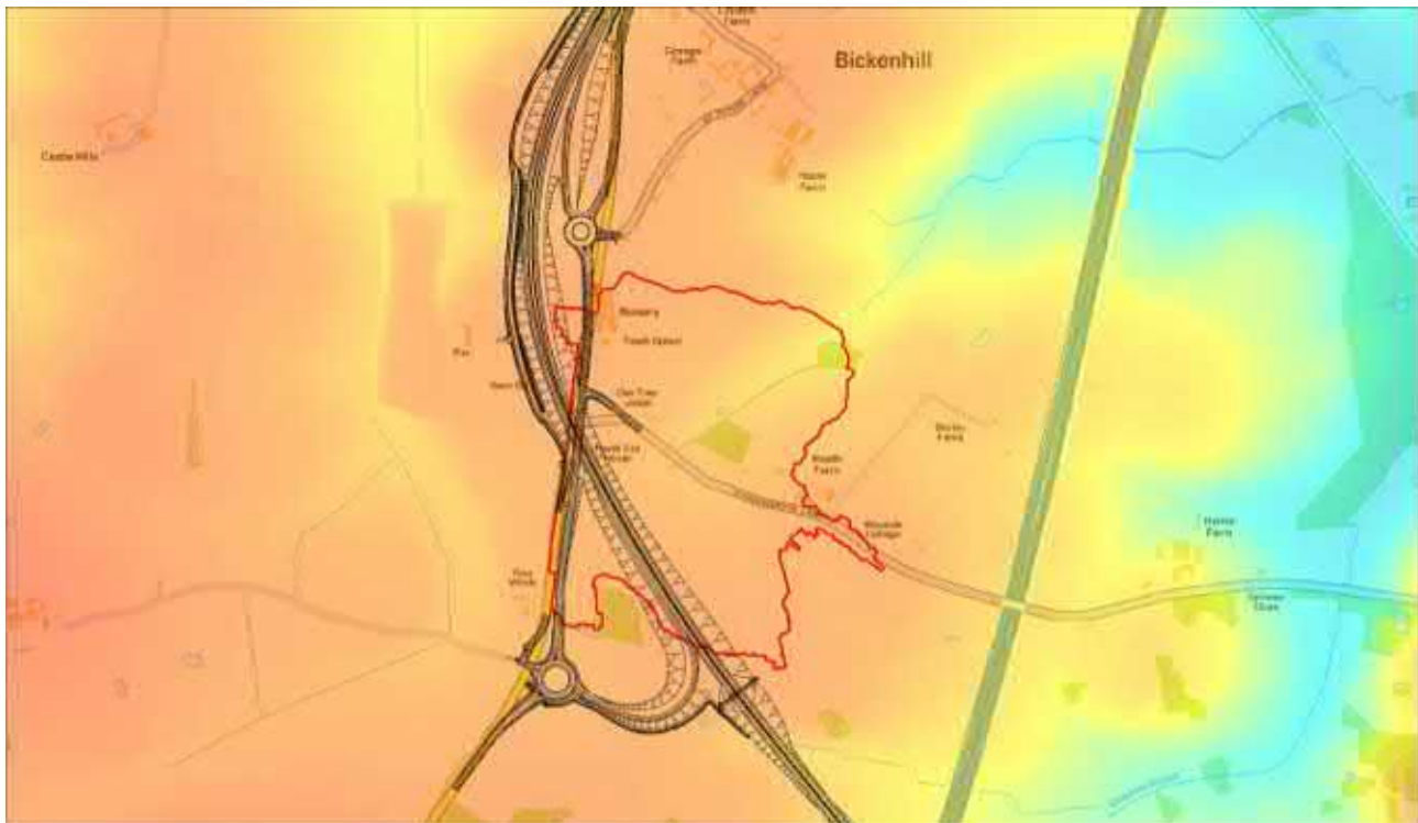
Figure 2: LiDAR data showing the elevation of land in the catchment area contributing to the SSSI
