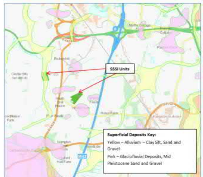
Figure 5. Superficial deposits in the area around Bickenhill Meadows SSSI (source: British Geological Survey Geindex website, http://www.bgs.ac.uk/geindex ).
