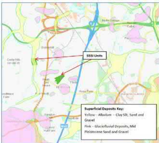
Figure 5. Superficial deposits in the area around Bickenhill Meadows SSSI (source: British Geological Survey Geindex website, http://www.bgs.ac.uk/geindex ).
