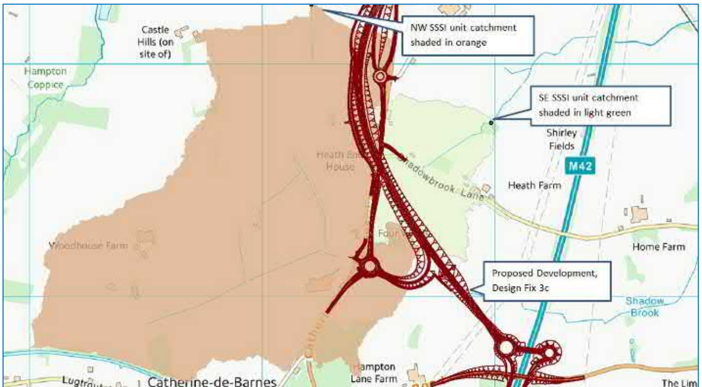
Figure 8. Catchment boundaries as determined from GIS catchment analysis, with the Design Fix 3C road alignment overlain in red.
