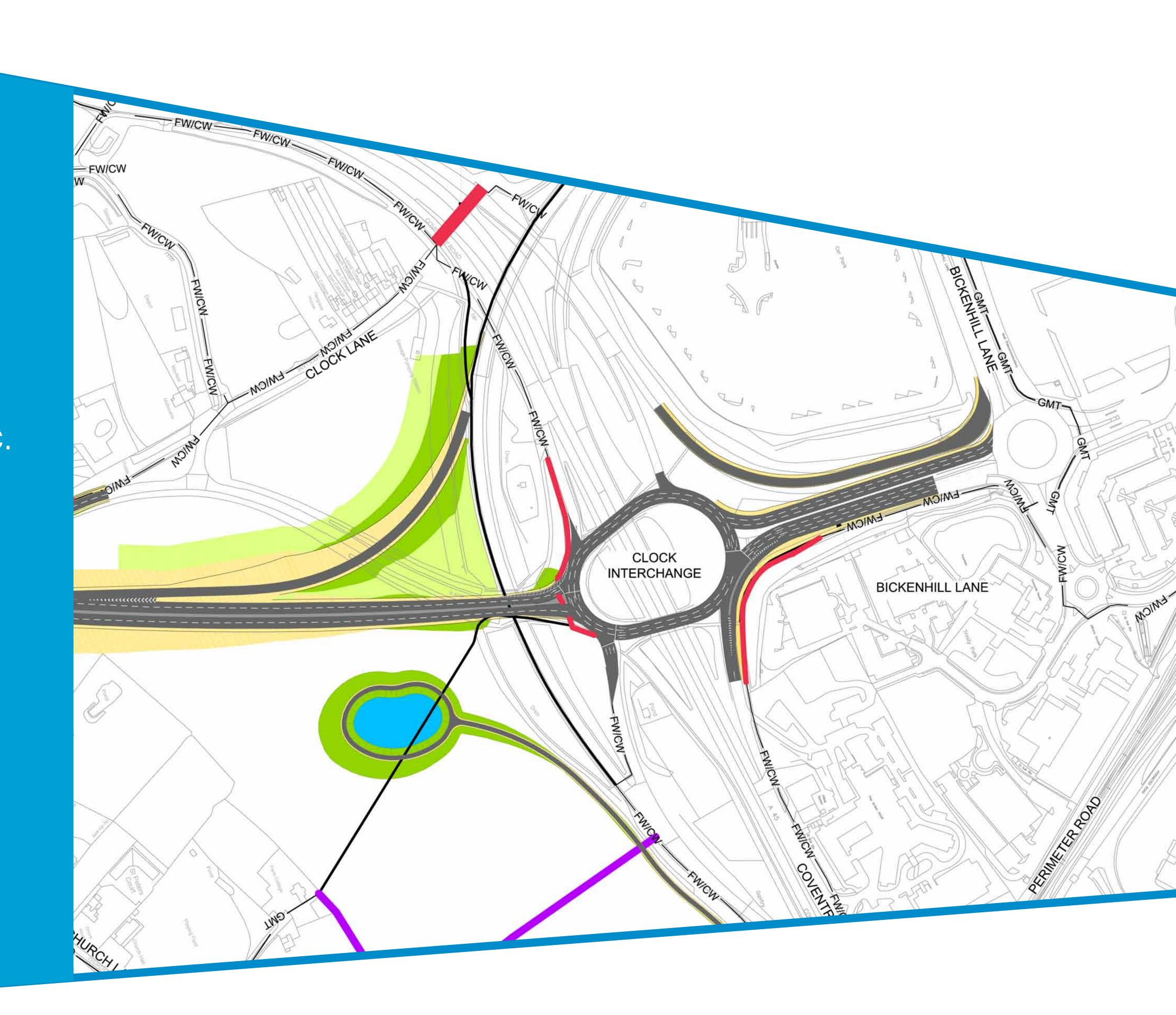
In addition to the link road, there will be two dedicated left-hand links around the M42 junction 6, reducing the number of vehicles having to use the roundabout.
