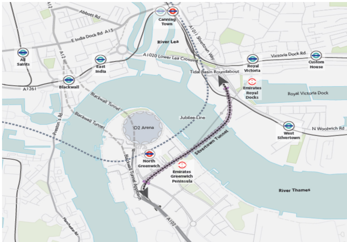
Figure 2-1 The alignment of the Silvertown Tunnel
