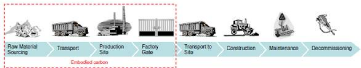
Figure 11.3: Diagrammatic representation of the measure of embodied carbon in relation to material life cycle
