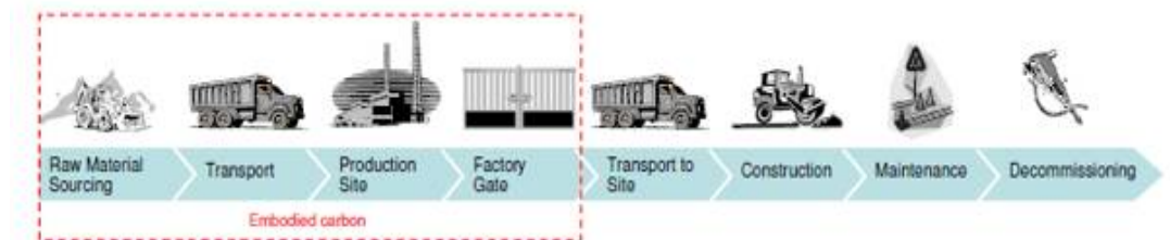
Figure 11.3: Diagrammatic representation of the measure of embodied carbon in relation to material life cycle
