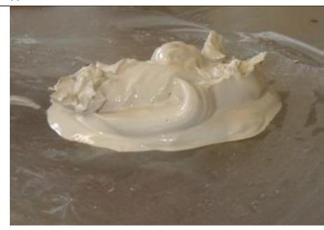
The use of centrifuges and filter-presses would significantly improve spoil consistency, and should result in chalk "cakes" with a moisture content of <30% (typically a M/C of 26% is aimed for) as shown below;
