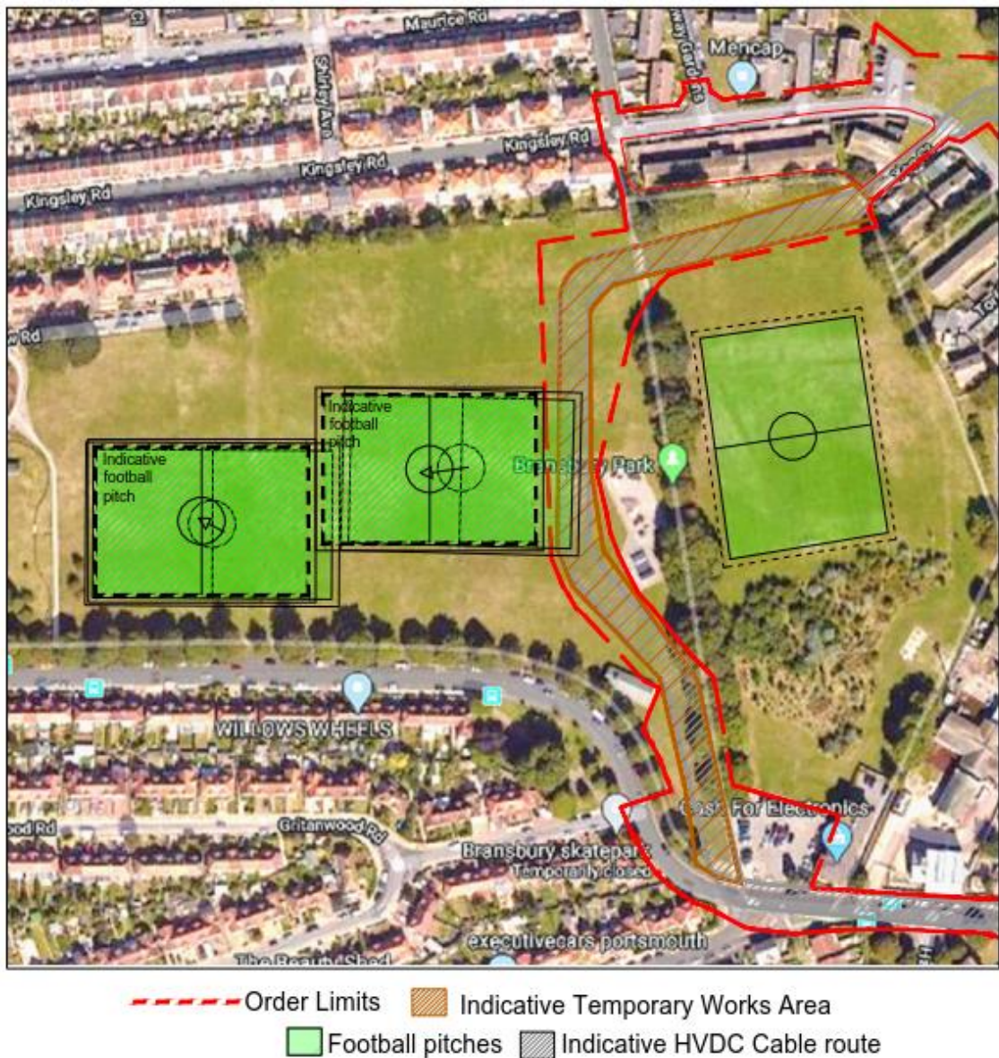
Plate 7 - Bransbury Park, indicative construction layout
