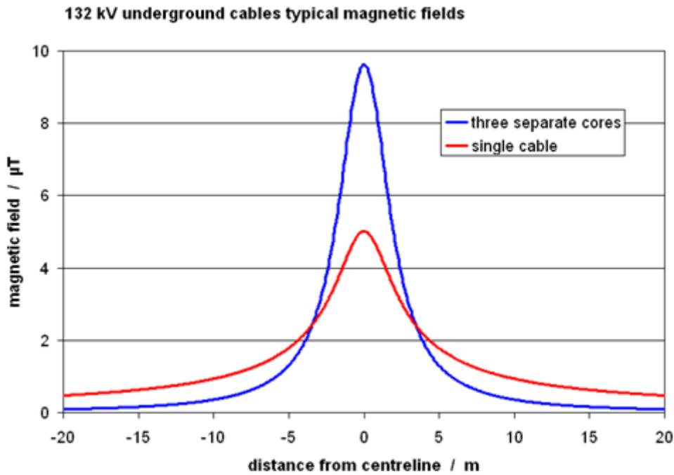
14.9.6 Underground cables do not produce any external electric fields. Table 14.5 gives some actual magnetic field values for the same conditions with fields calculated at 1m above ground.
