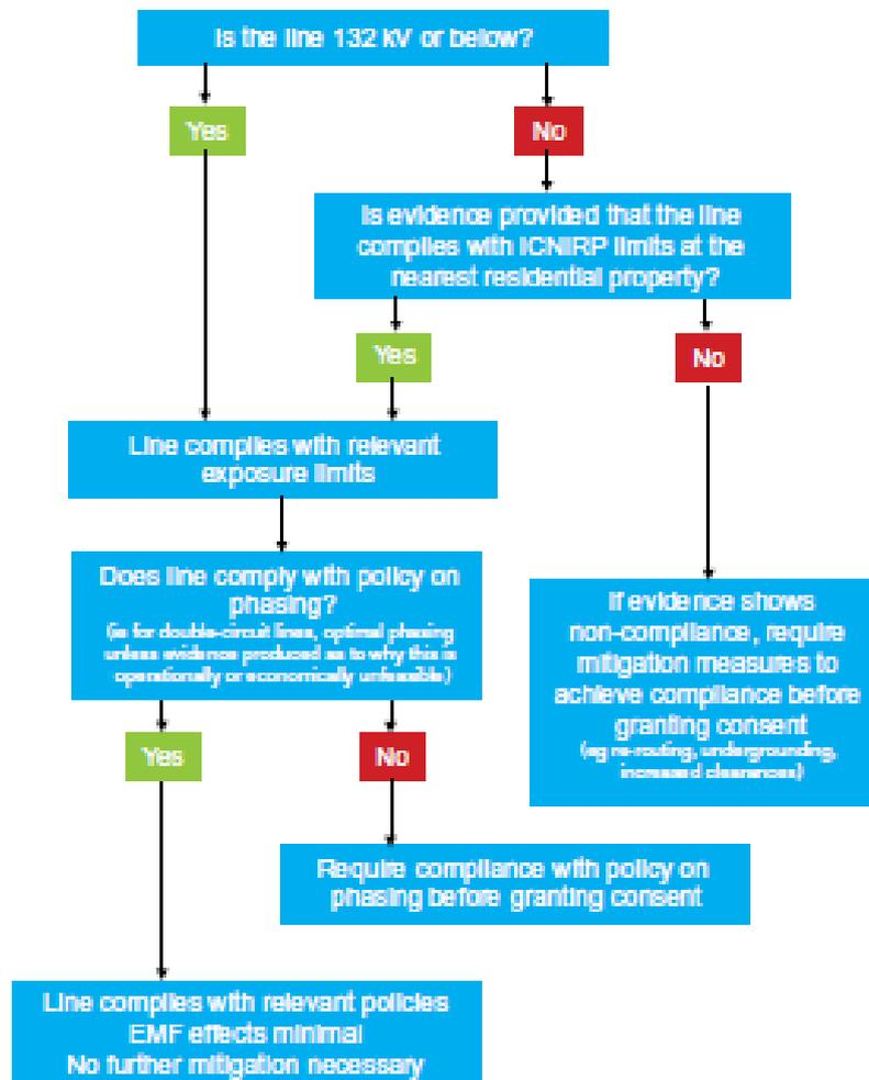
14.2.8 NPS (EN-5) does not require evidence to be provided for 132 kV or below overhead lines as they are deemed to comply with relevant exposure limits. The Proposed Development includes a single-circuit overhead line and therefore optimal phasing is not relevant. SP Manweb has carried out calculations on the potential levels of EMFs to provide evidence to show that the line complies with the ICNIRP limits.
