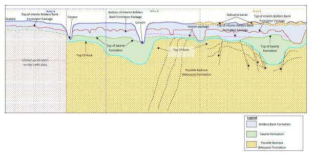
Figure 1. Schematic of interpreted units within the Outer Dowsing array area (west - east) (Enviros, 2022)
