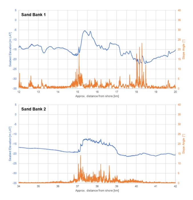
Plate 7.7 Bathymetric and gradient profile along the offshore ECC at the Inner Dowsing (Sand Bank 1) and North Ridge (Sand Bank 2) sandbanks, as labelled in Figure 7.15. Data from Project Cable Burial Risk Assessment (CBRA).
