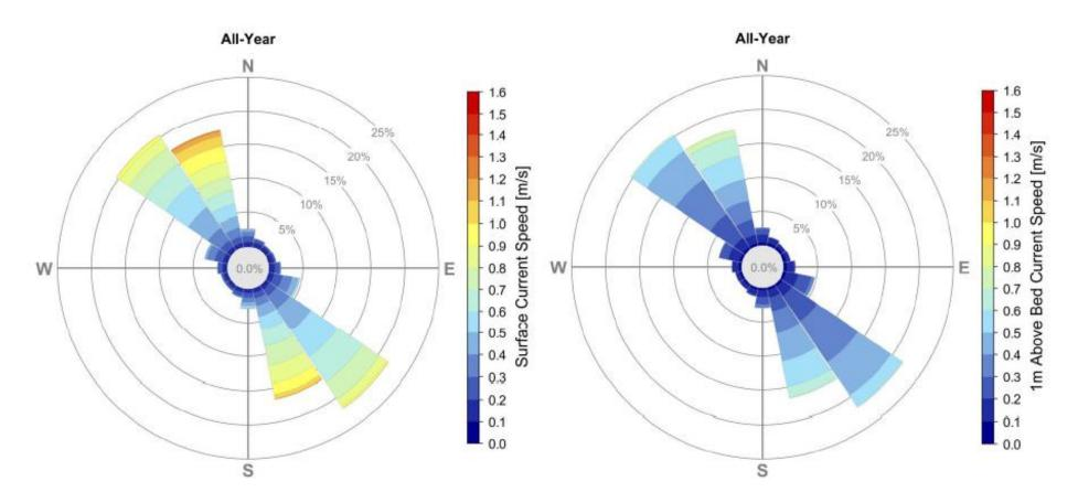
Plate 7.3 Annual rose plot of modelled surface and near bed current speed and direction in the centre of the array area (MetOceanWorks, 2021b)
