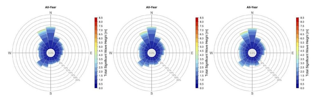
Plate 7.1 Array Area annual wave rose for Hm0 and direction at the three model points (from left to right: West, Central, and East, as shown on Figure
