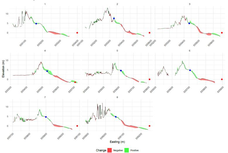
Plate 7.11 Difference plots between LiDAR data across the dune and beach frontage between 2016 and 2020, with transect locations shown in Figure 7.20. MHWS and MLWS are indicated by the blue and red dots, respectively.
