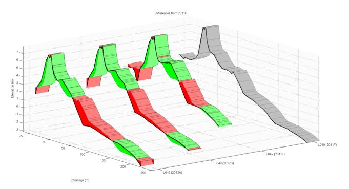
Plate 7.10 Difference in the beach profile at transect L049 (see Figure 7.17) over the last three surveys compared to the beach in June 2011. Lowering is shown in red (Environment Agency, 2013a)
