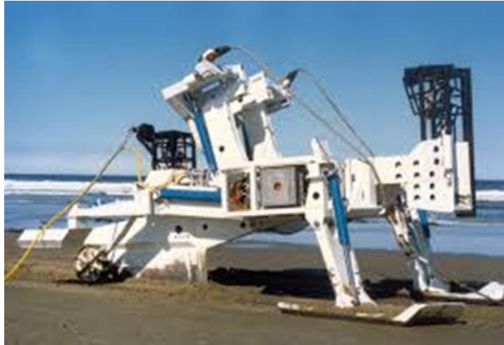
Graphic 4-14 Typical marine cable installation plough
