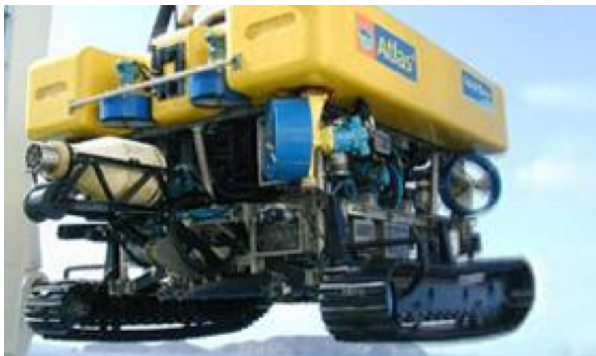
Graphic 4-16 Typical marine cable jetting seabed fluidiser
