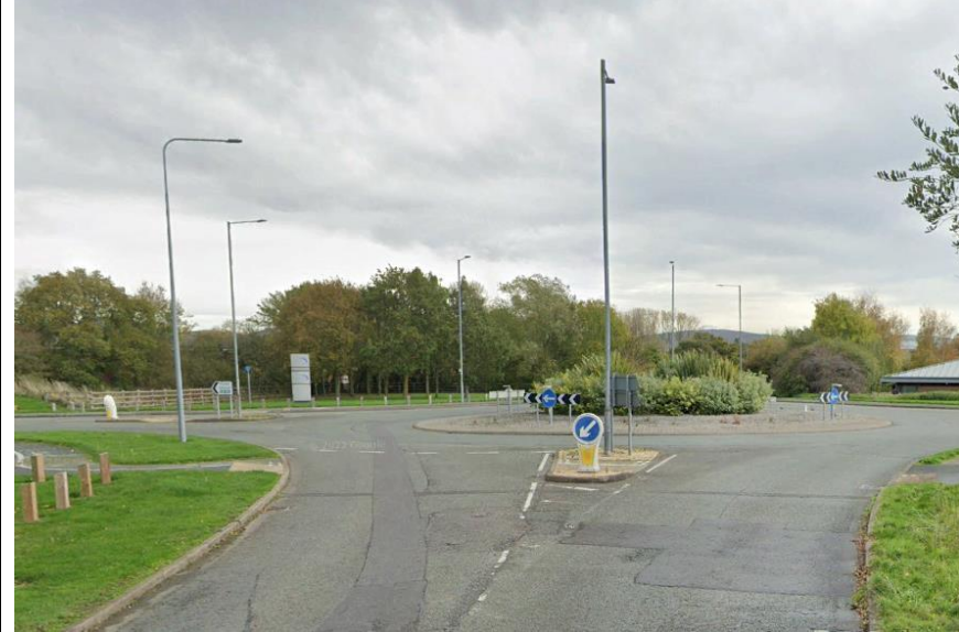
Picture 14. St Asaph Business Park/B5381 Glascoed Road roundabout. On route 3, loads turn right at this roundabout which for 20 axle frame trailers would be best undertaken in contraflow. Caution is required in relation to lamp posts and street furniture but the turn is considered negotiable.
