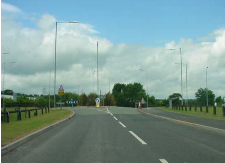
Picture 10. St Asaph Business Park Roundabout. Load moves away from camera. For possible site entrance 2 load turns left. For alternative access to possible site entrance 3 (see section 3.3) load continues straight over roundabout.
