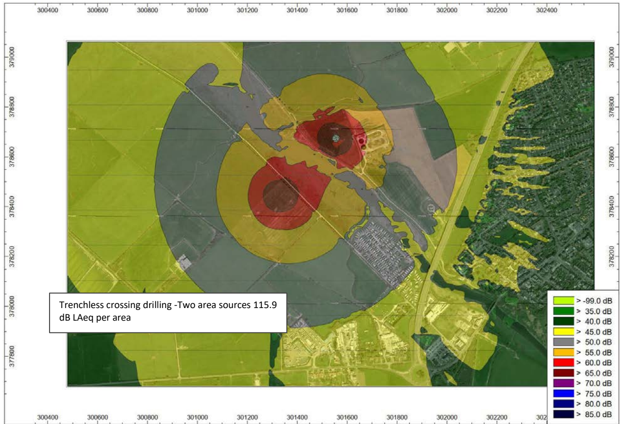
Figure 3-4 Model 2 – Trenchless crossing Drilling at the River Clwyd Crossing with Mitigation Included
