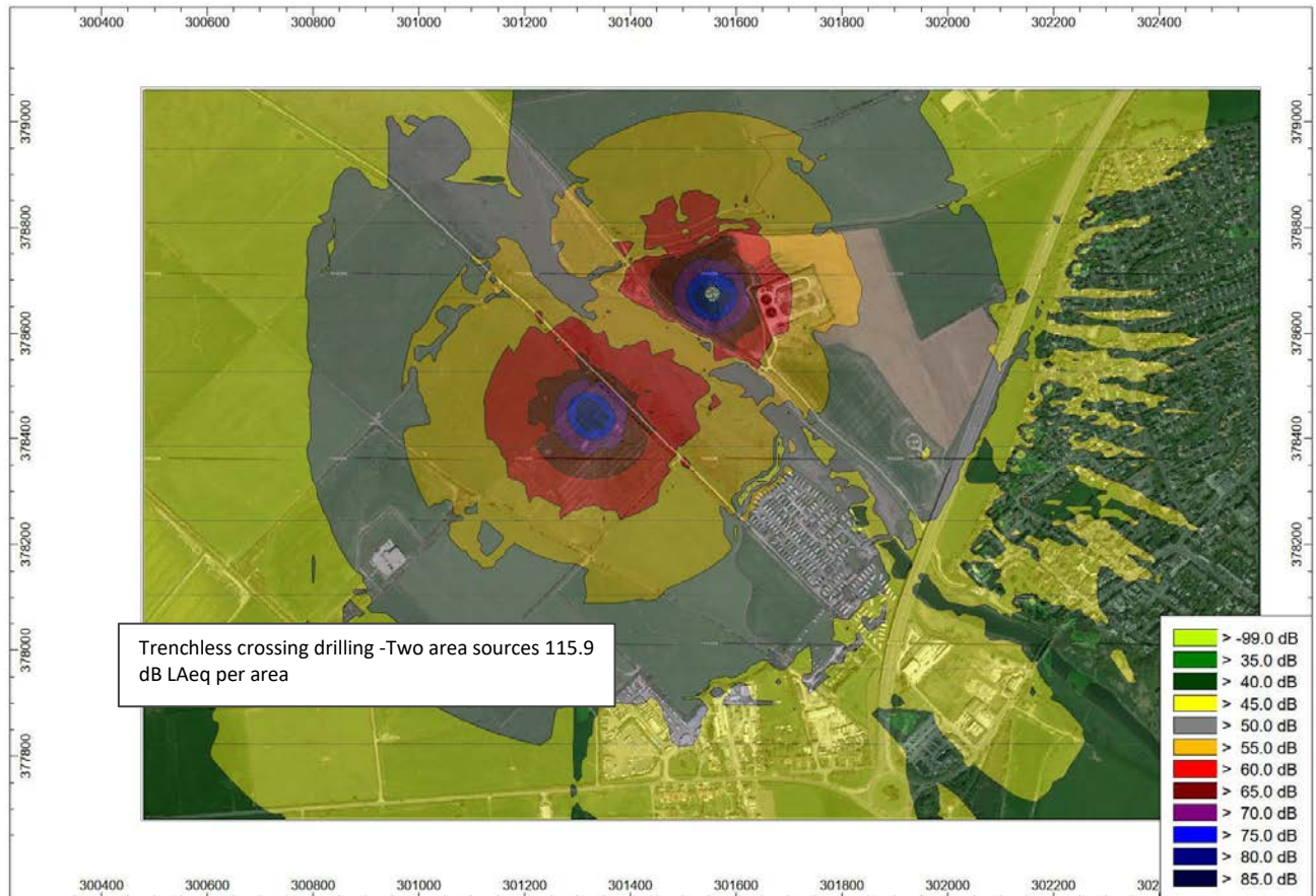
Figure 3-3 Model 1 – Trenchless crossing Drilling at the River Clwyd Crossing (Unmitigated)
