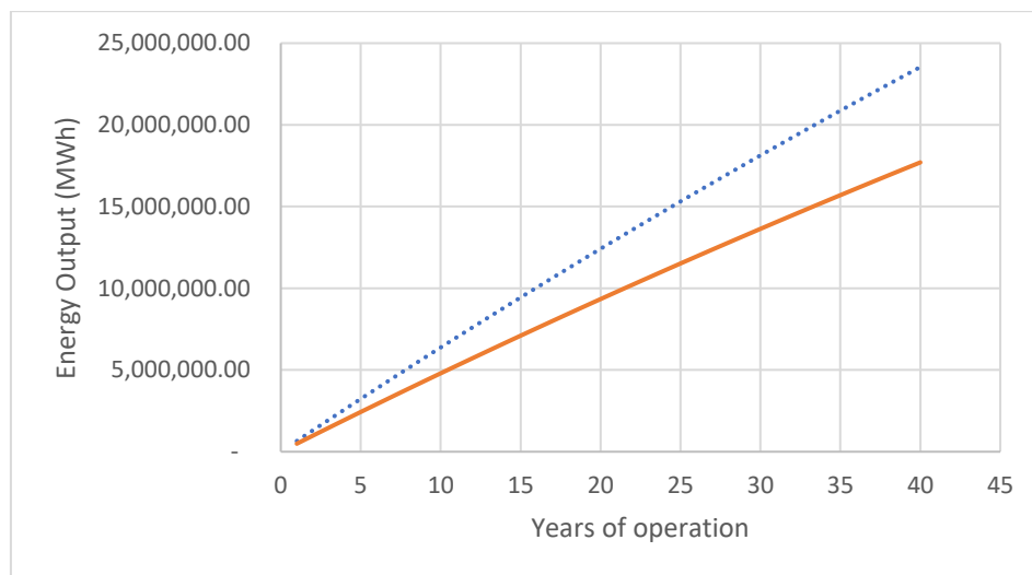
Figure 2 Total Energy from Plant (comparison between Sunnica's estimates and recalculated values based on more realistic estimate for energy output in 1 st year of operation obtained using Global Solar Atlas)
