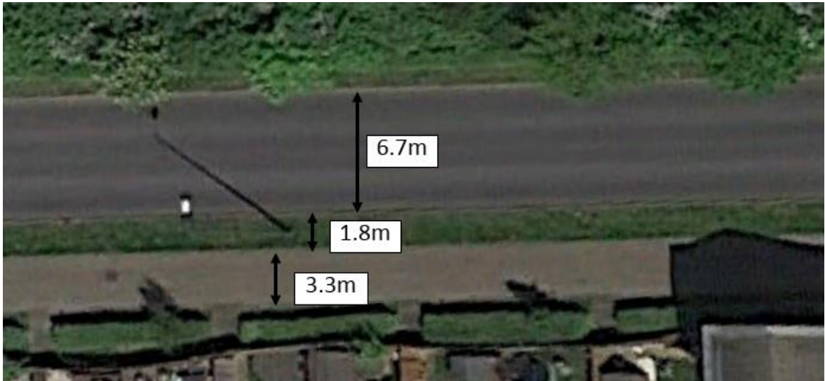
Figure 4: Typical Corridor Widths
