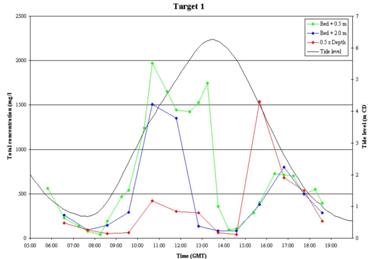
Figure 4.1: Suspended fine sediment concentration observed near the Power Station Jetty in July 2002 (HR Wallingford, 2002).
