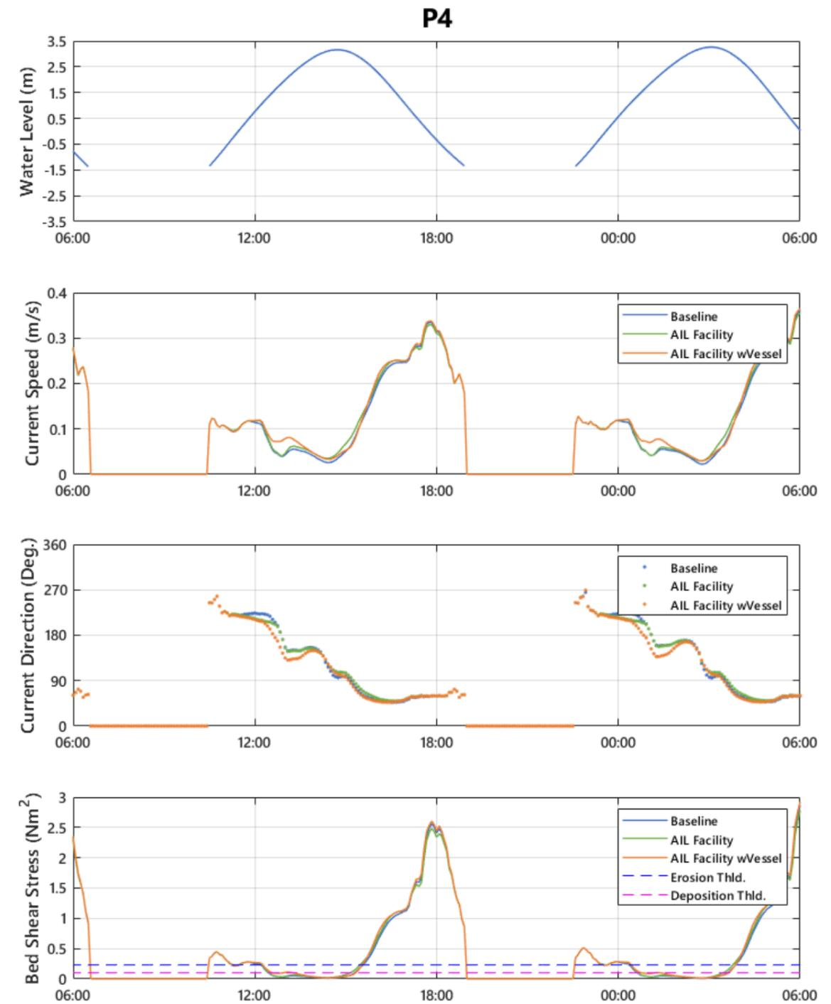
Figure 3.6: Comparison of current speed, direction and BSS as a result of the AIL Facility and AIL Facility with RoRo vessel compared to the baseline at P4.
