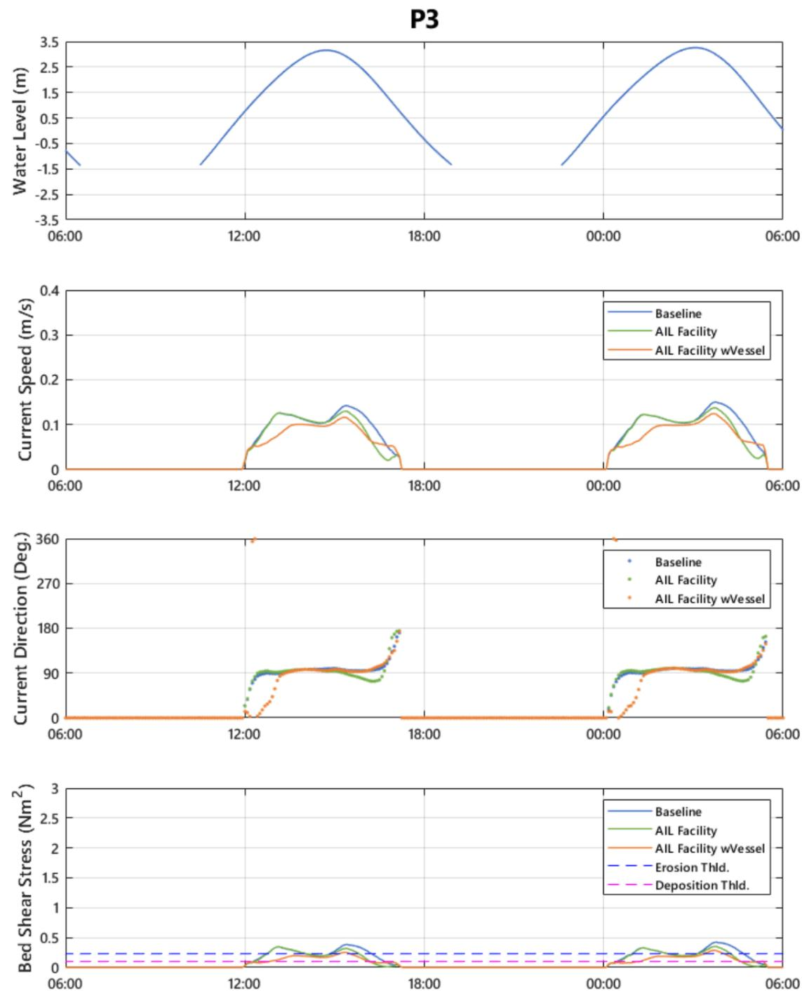
Figure 3.10: Comparison of current speed, direction and BSS as a result of the AIL Facility and AIL Facility with RoRo vessel compared to the baseline at P3.
