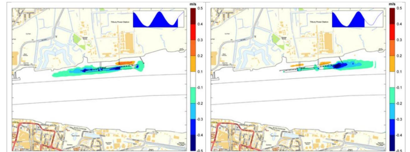
Figure 3.11: Effect of Tilbury2 scheme with 3 vessels on flow speeds during peak flood (left) and peak ebb (right). HR Wallingford, 2017.
