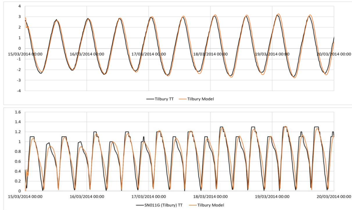
Figure 2.7: Comparison between modelled and TT water level (top) and flow speed data (bottom) at Tilbury.
