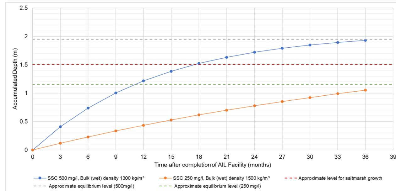
Figure 4.2: Accumulated depth over a 3-year period for SSC of 250 mg/l, bulk (wet) density of 1500 kg/m<sup>3</sup>; and SSC of 500 mg/l, bulk (wet) density of 1300 kg/m<sup>3</sup>.
