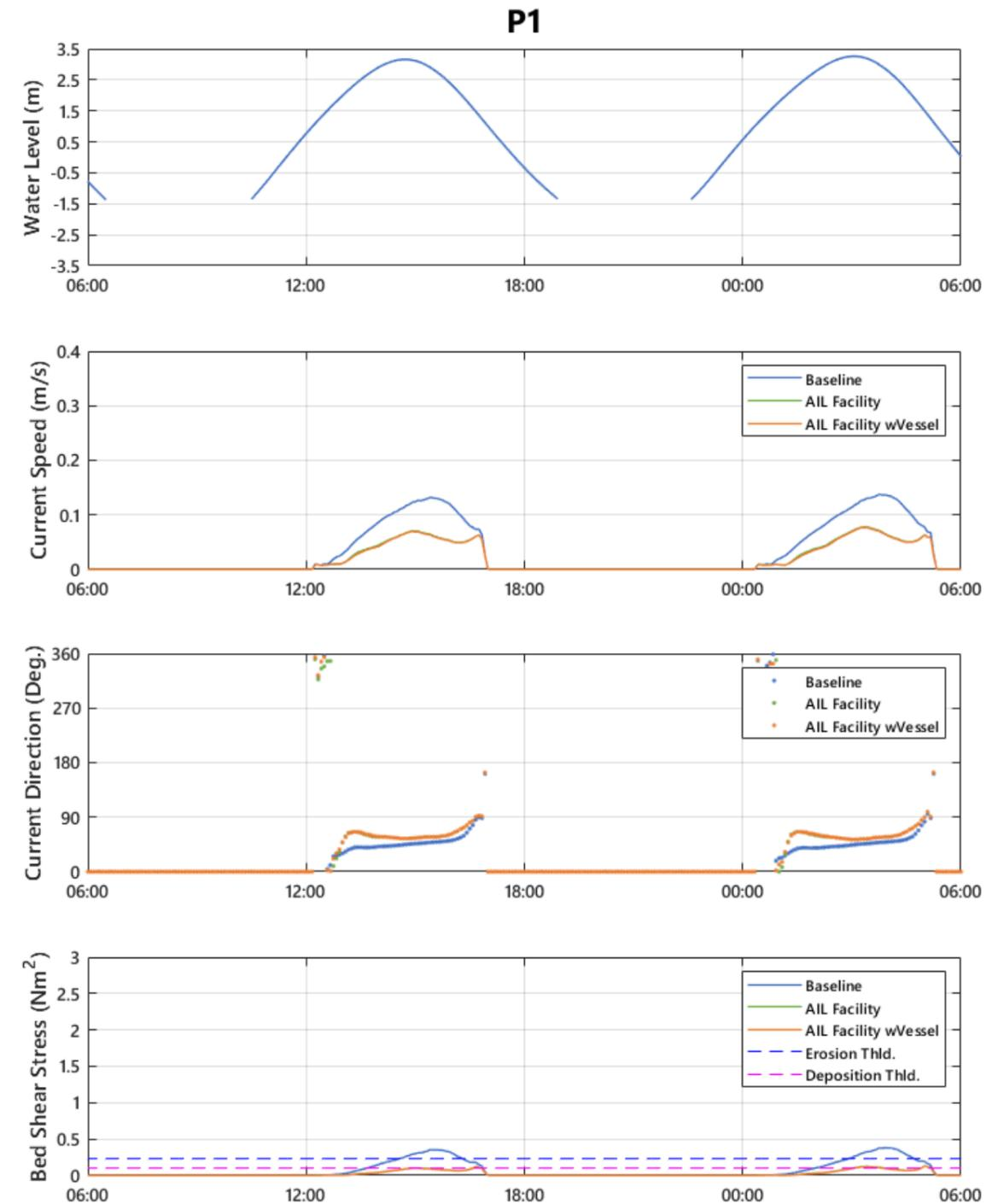
Figure 3.3. Comparison of current speed, direction and BSS as a result of the AIL Facility and AIL Facility with RoRo vessel compared to the baseline at P1.
