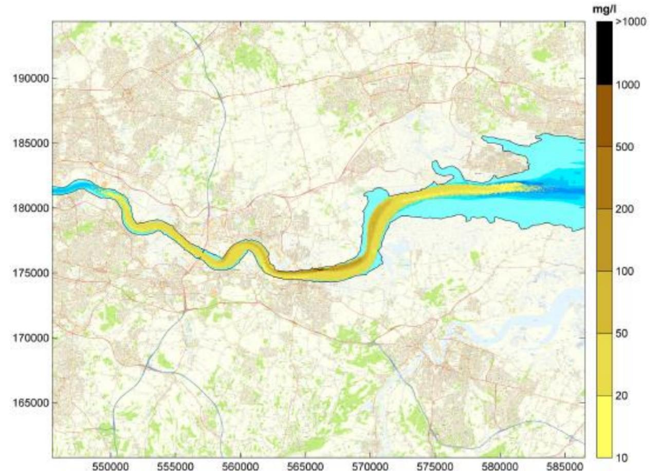
Figure 5.1: Maximum increase in depth averaged suspended sediment concentration during 14 days of WID - Scenario 1 (HR Wallingford, 2017).
