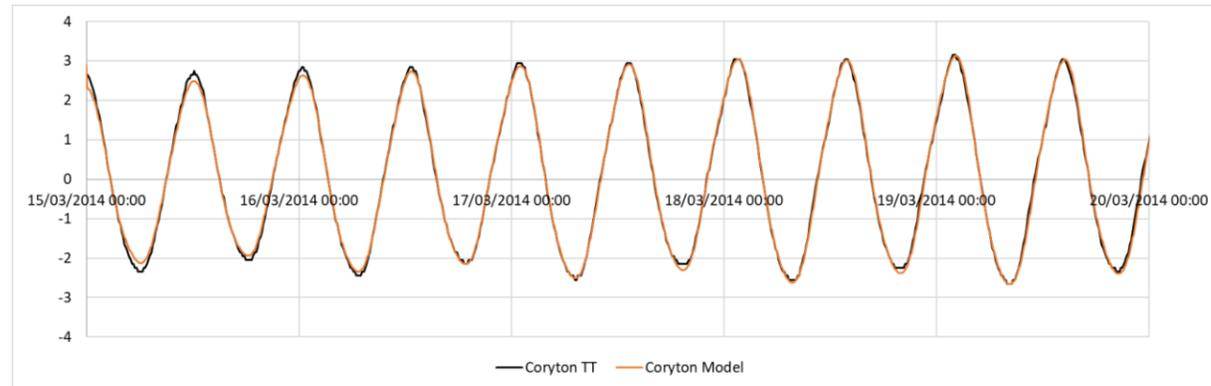
Figure 2.6: Comparison between modelled and TT water level data at Coryton.
