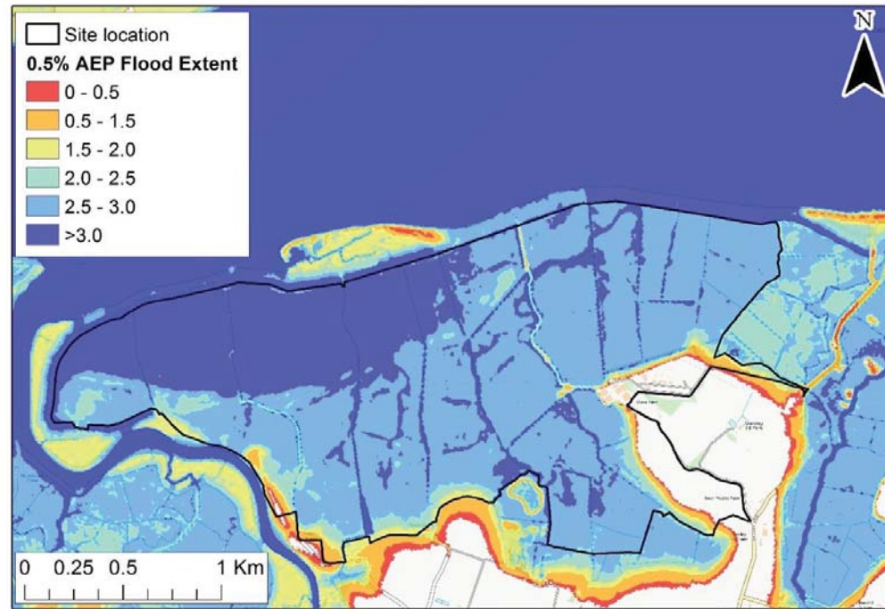
Figure 3-6: Undefended - 0.5% AEP present day flood depth
