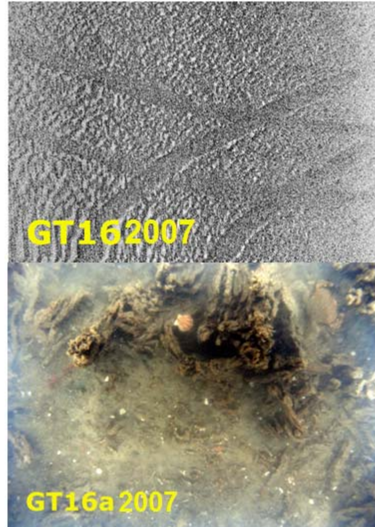
Plate 11. Example of the raw, high resolution, Side Scan Sonar data and seabed imagery taken at ground-truth station GT16 within the TOWF site in 2007. This station showed clear damage from trawling.
