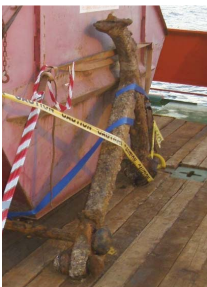
This anchor was recovered during cable installation for a wind farm. It is probably a Rodgers' Small-palm anchor, named after Lieutenant (later Commander) Rodgers and was patented in 1832. The anchor was carefully recovered to the vessel, recorded and reported, and returned to the seabed away from development impacts.
