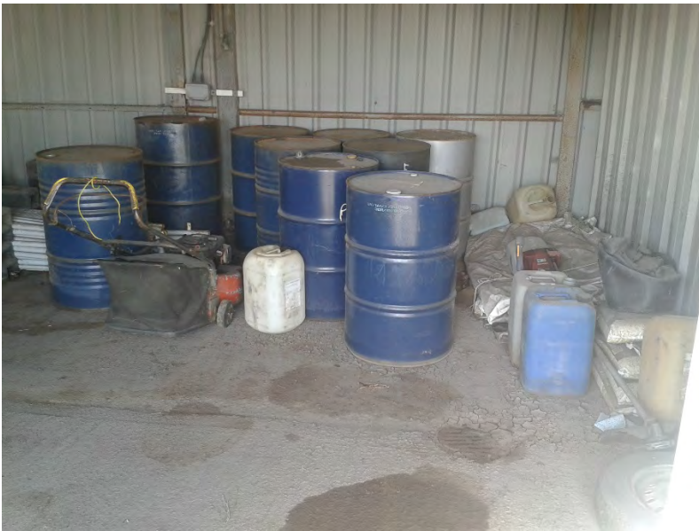
Picture 19 Storage with signs of spillages
