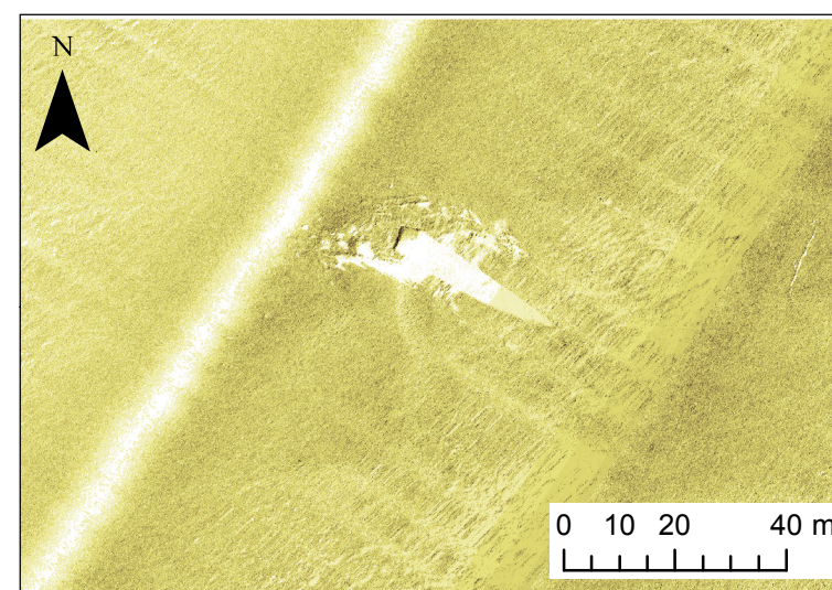
Sidescan sonar image of wreck 70219, 44.1 x 32.6 x 3.8 m
