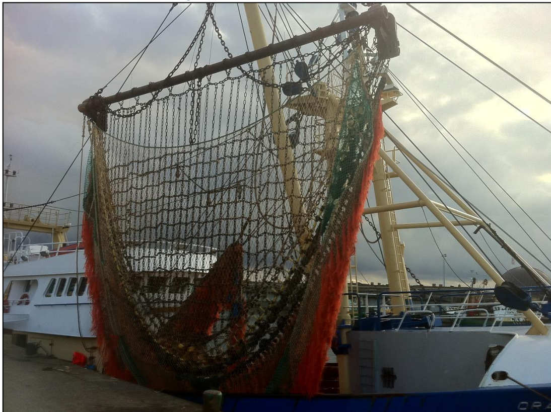
Plate 3.3 Traditional beam trawl with tickler chains and chain mat (source: BMM, 2012)
