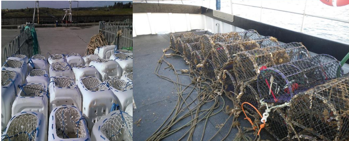
Plate 3.1 Whelk pots (left) and “parlour” pots (right) used to target whelks and lobsters (source: BMM 2016, 2013)
