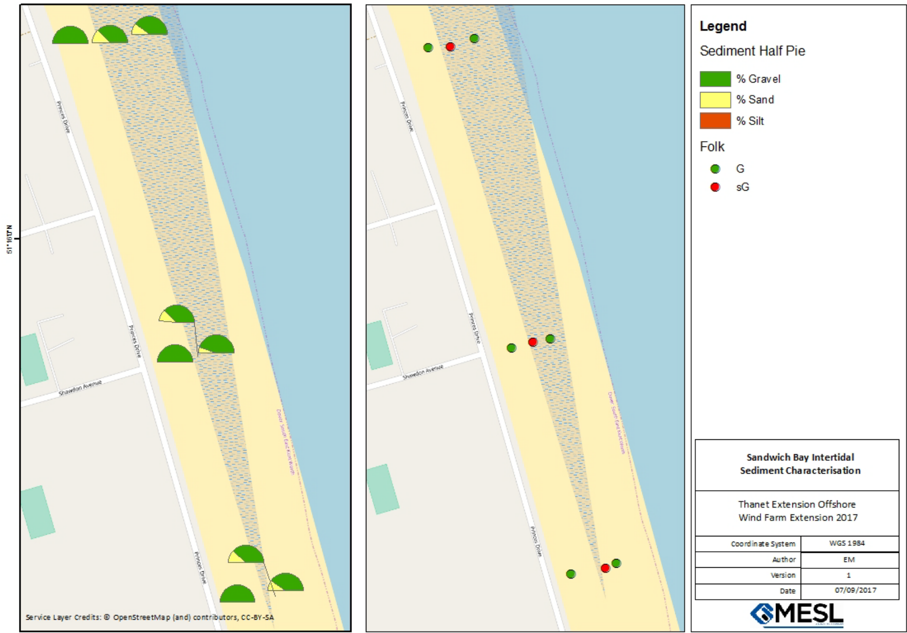
Figure 7. (left) The relative proportions of gravel, sand and silt in the PSA samples obtained across Pegwell Bay. The location of the diagrams represents approximate station positions. (Right) PSA samples classified using the Folk classification system
