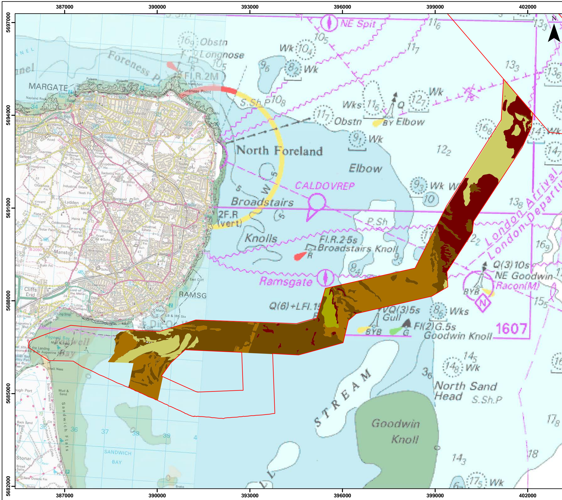
Figure 3.5 Sediment Classification from Site Specific Surveys in the OECC.
