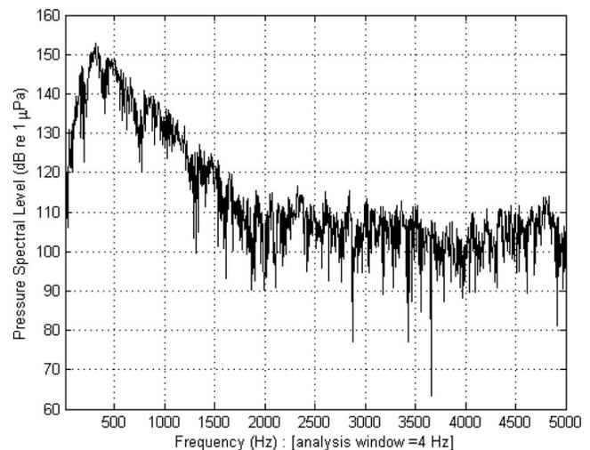
FIG. 6. Frequency spectrum analysis of the recorded airgun impulse (Fig. 4) showing the pressure spectral level (dB re 1  $\mu\text{Pa}$ ). The frequency spectrum is plotted in hertz, and the spectrum levels are based on a 4 Hz analysis band.
