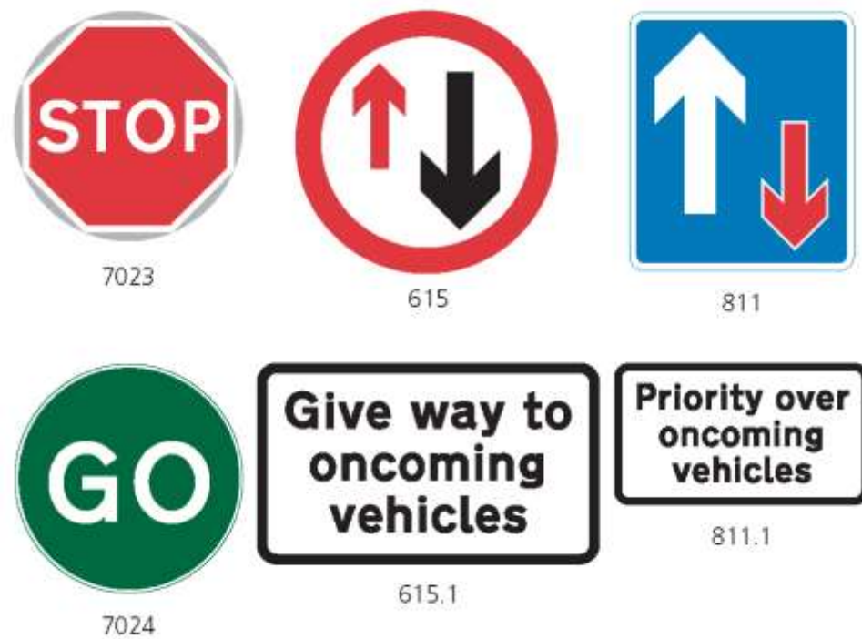
Figure 3.5: Manually Operated Stop/Go Signs and Priority Signs.
